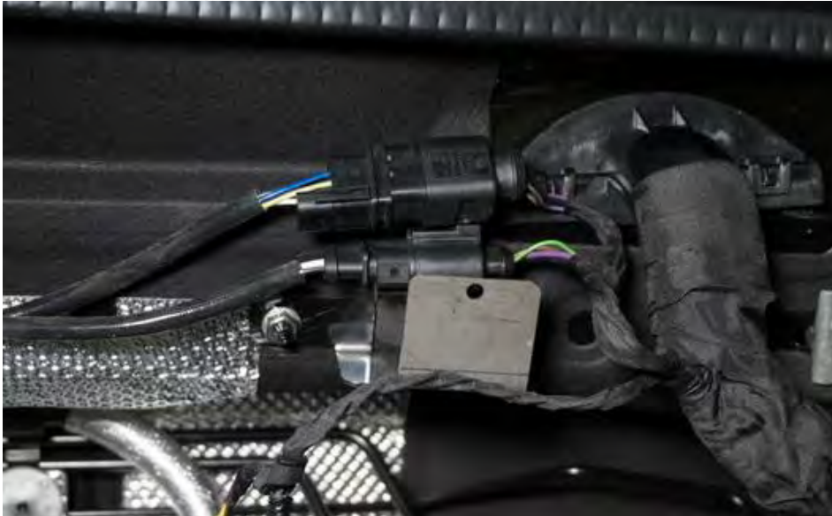
13. Install the new bracket onto the threaded stud as shown and secure with the supplied M6 Nut.
