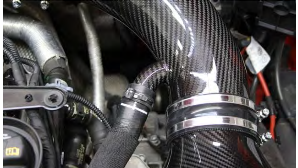
38. Push the breather onto the carbon tube and secure with the original spring clamp.
