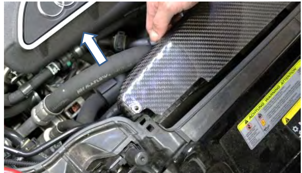
20. Push the hose shown away slightly to allow the left side of the duct to be positioned into place. Lower the duct and place into the mounting area as shown in next step.
