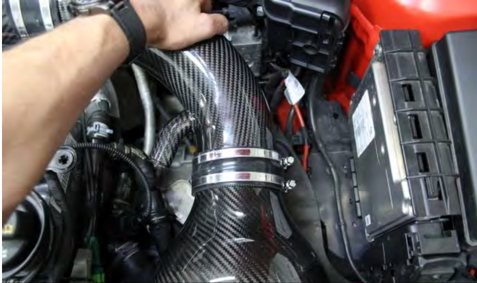
37. Tighten the remaining hose clamps between the lower tube and housing. Ensure the clamps are evenly positioned. Do not over tighten.
