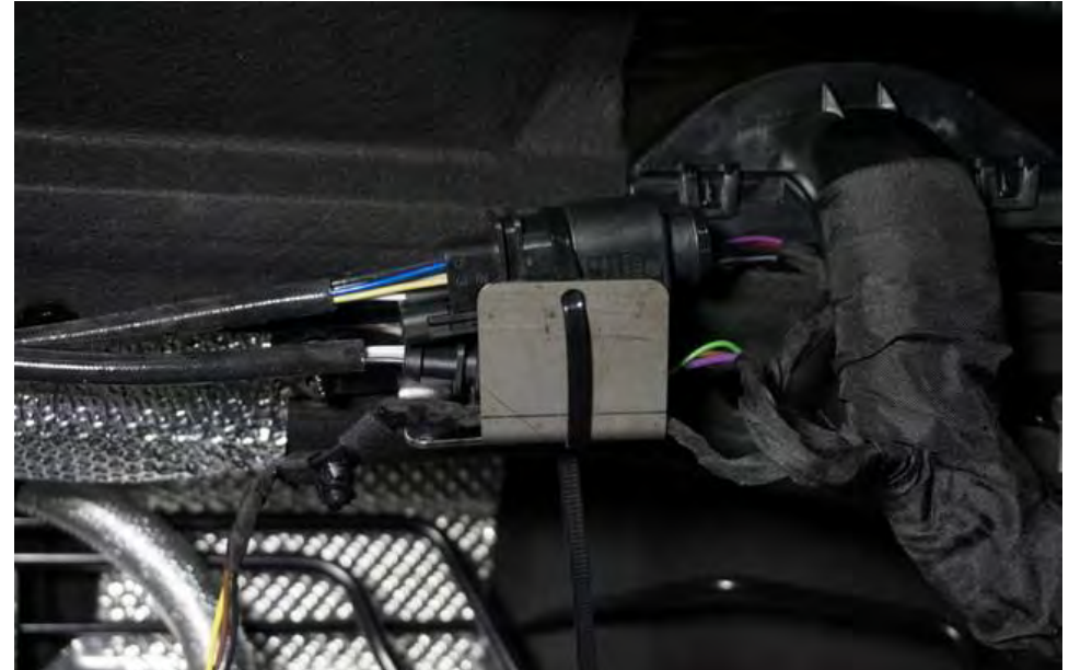
14. Place the wiring plugs into the bracket and secure with a cable tie. Cut the excess off.
