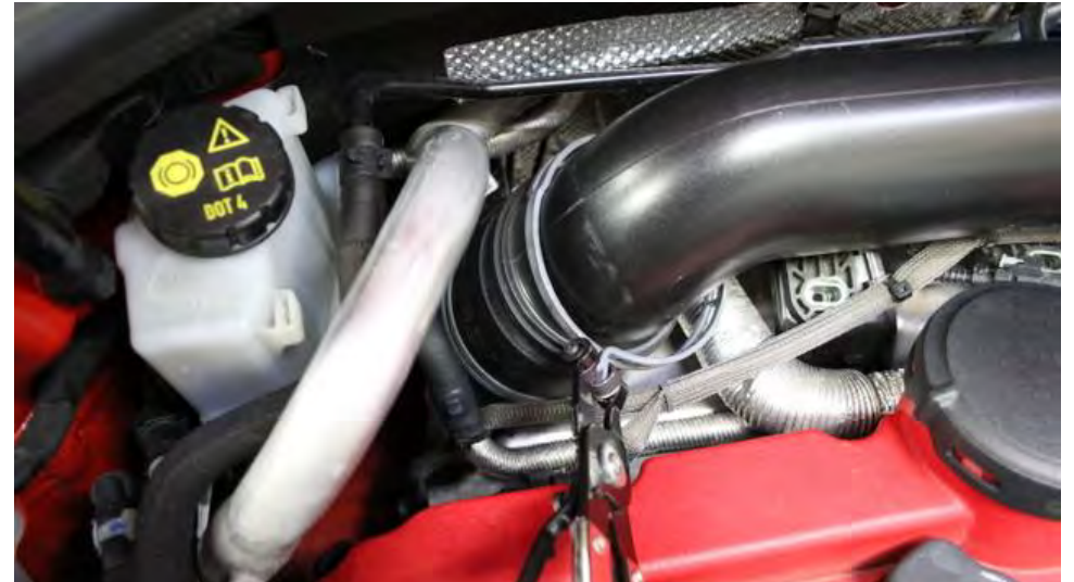
6. Remove the spring clamp holding the turbo tube to the rubber joiner and pull the tube out.
