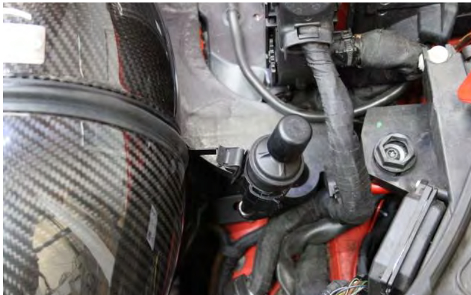
39. Push the sensor pot onto the small bracket extending from the housing.
