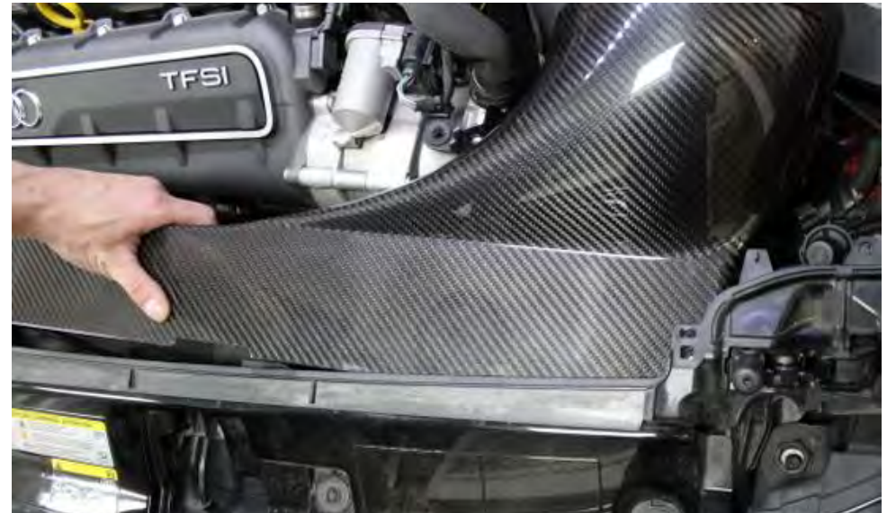
18. With the duct pushed as far as possible into the right of the mounting area – lower it and position the top surface of the carbon panel into the mounting area.
