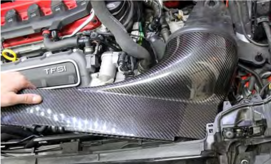
17. Carefully lower the duct as shown into the right side corner of the mounting area first. Don't line up the mounting hole yet – push it as far as possible to the right for clearance to lower it.
