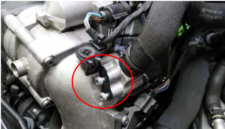
15. Remove the 2 Torx screws at the front of the engine on the inlet tube where the breather is also located. Pull the bracket off the mount.
