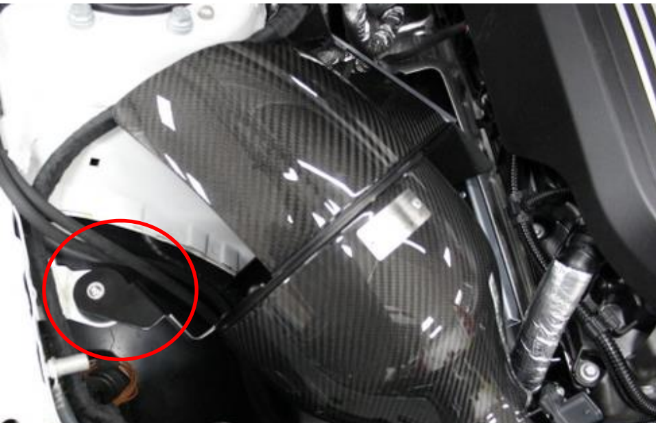
19. Push the mount on the housing bracket into the rubber stock mount
