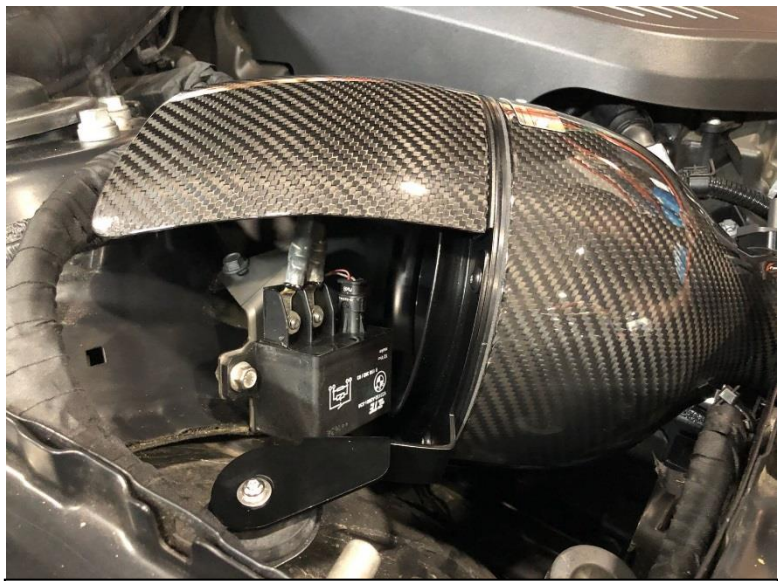
6. Once the intake is installed – the relay will sit in front of the filter.
