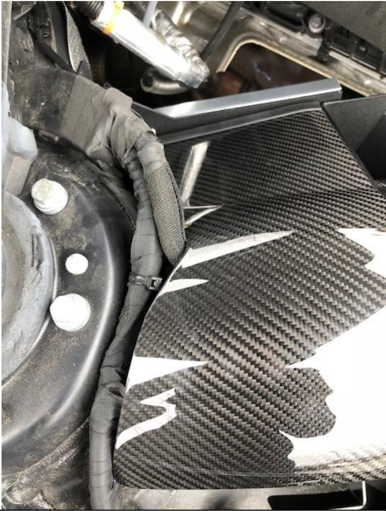
7. Position the relay loom through the cut-out in the carbon shroud.
