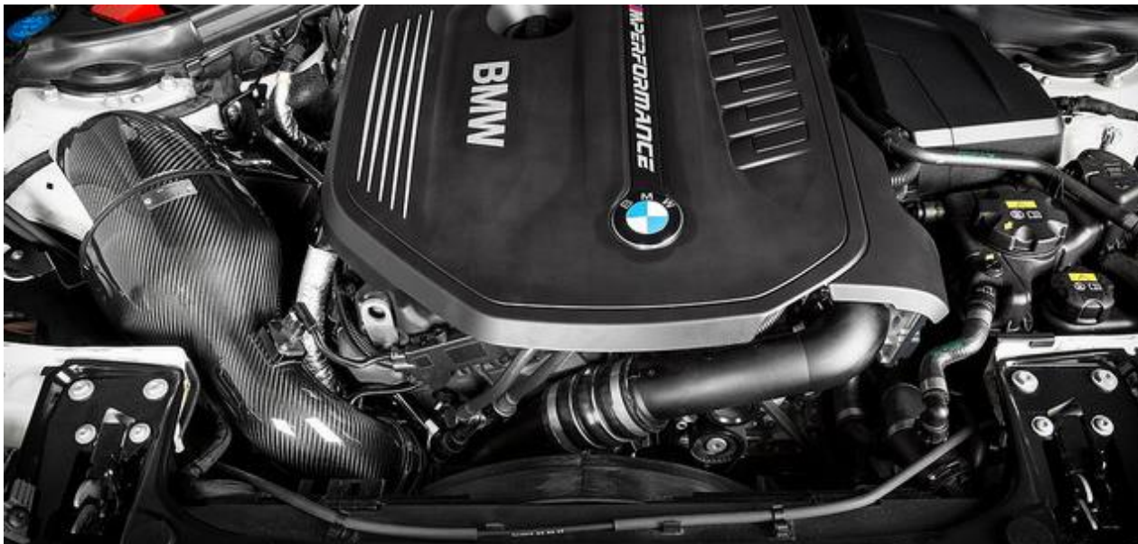
29. The scoop should sit as shown. The grill can now be pushed back into place.
