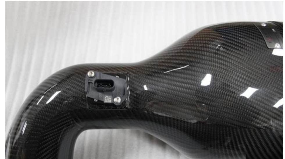
16. Install the sensor into the carbon intake as shown – the front hole of the sensor MUST face the filter. Secure with the 2 supplied M4 Torx screws.
