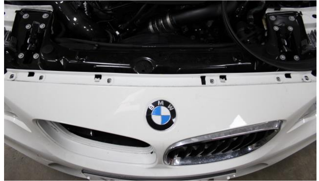
30. Secure the top of the bumper with the Torx screws and reinstall the rubber trim.
