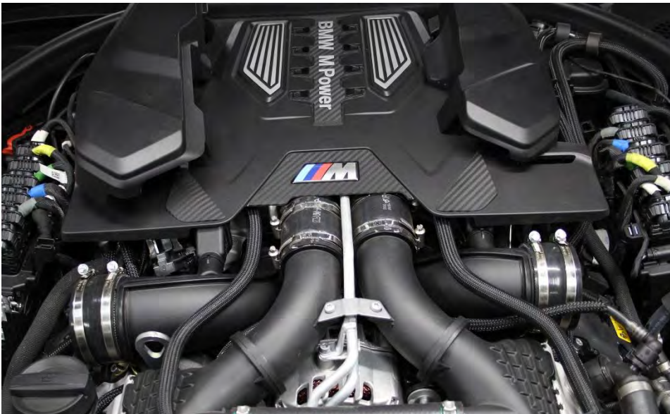
19. Push the 2 silicon couplers and hose clamps onto the turbo inlets. They should go onto the inlets as far as possible. Secure them by tightening the clamps around the inlets. Leave the other loose.
