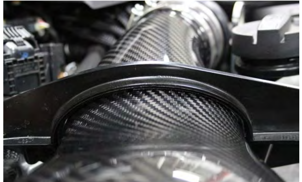
33. Now position the strut brace so that there is an even gap on both sides around the housing.
