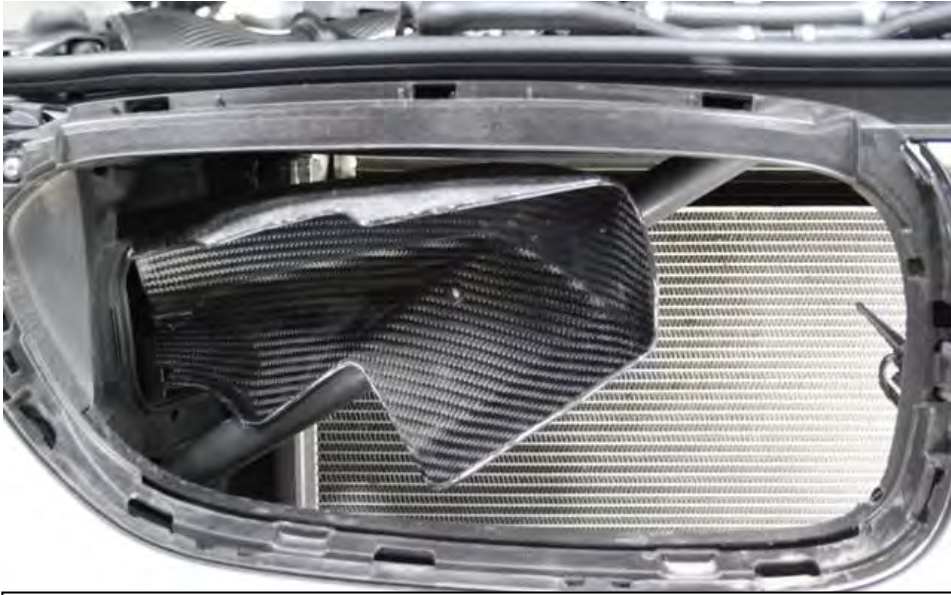
43. Push the scoop onto the bar so that the clip snaps over it.
