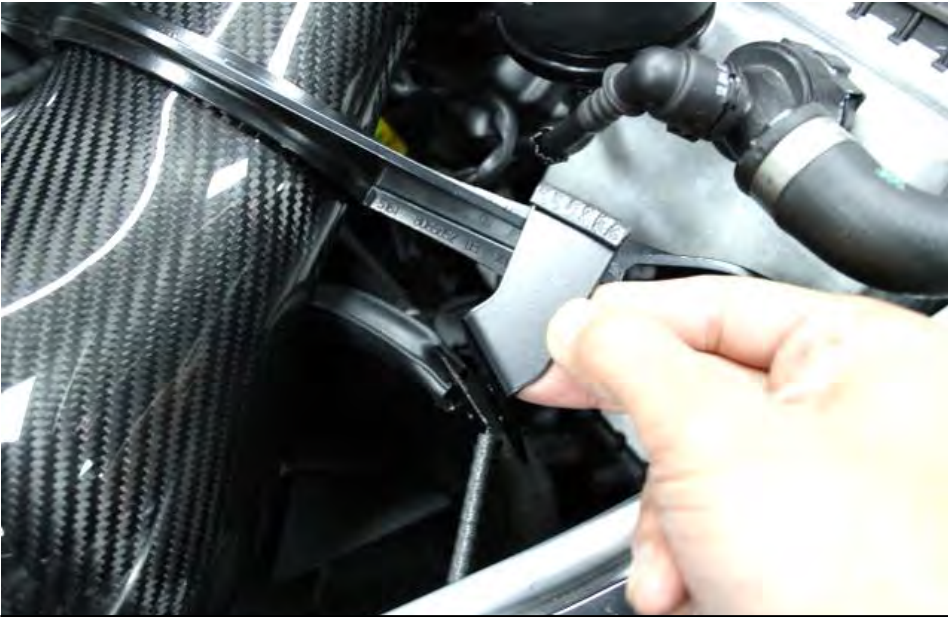
35b. Take the LHS bracket and position it between the LHS shield and strut brace.
