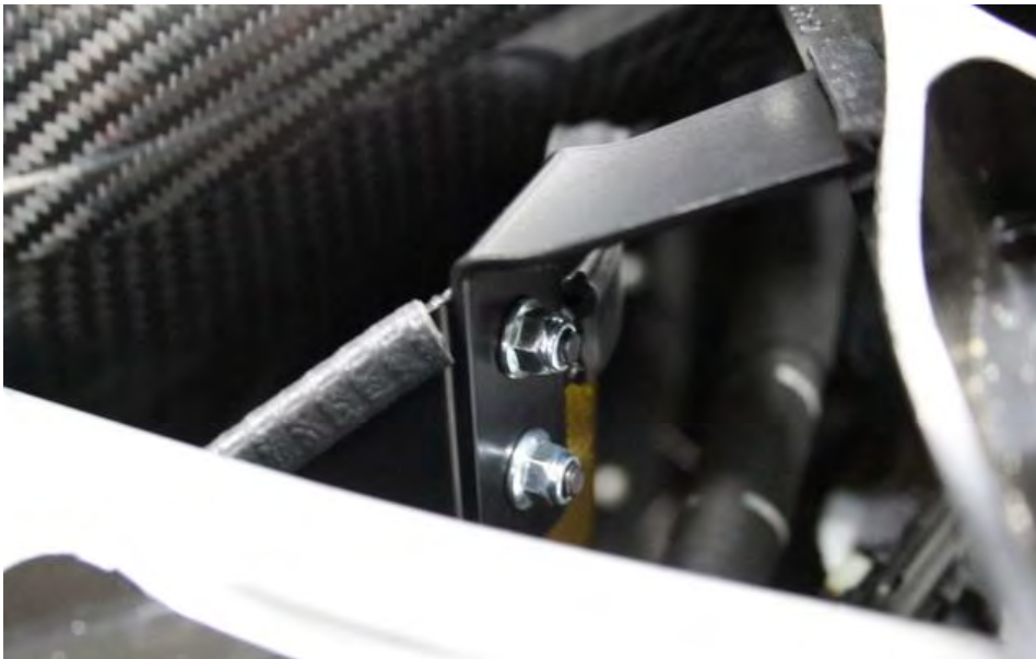
37. Another view of the secured LHS bracket.
