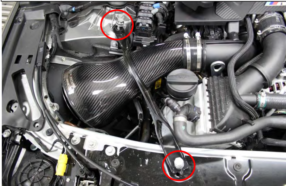
30. Insert the bolts through the strut brace but don't tighten yet. LHS Housing shown.
