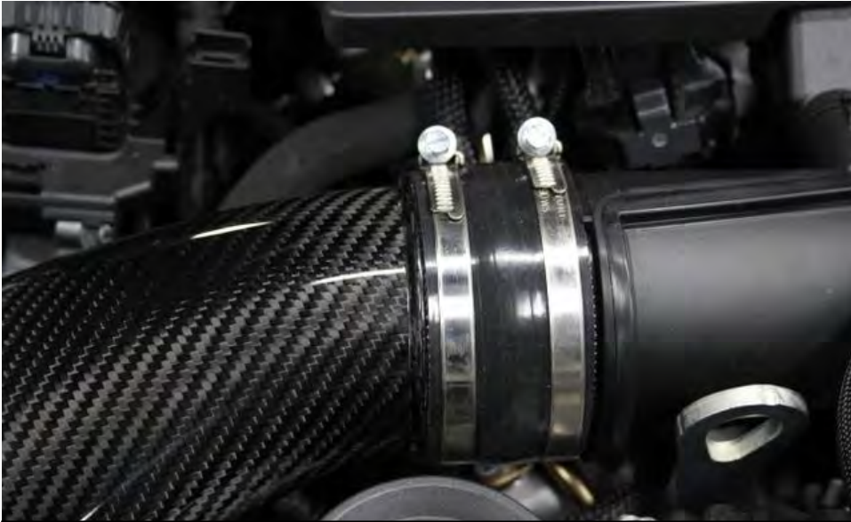
32. Once lined up – ensure that the carbon flange at the silicon end is squarely touching the silicon all around and tighten the hose clamp – do not over-tighten.
