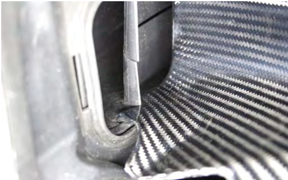
45. The start of the scoop should locate into the trim opening as shown.
