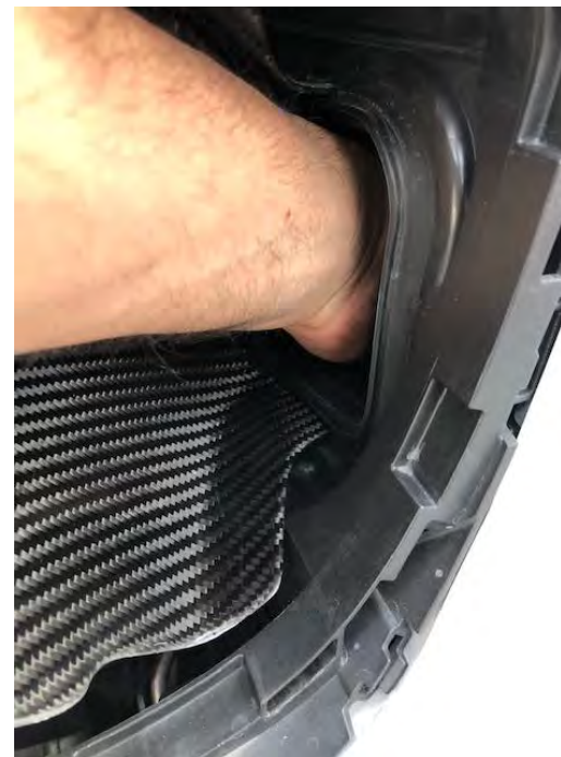
20. The inner duct panel may come loose as you push the clips in – pull the panel towards the scoop to ensure it secures with the scoop clips.
