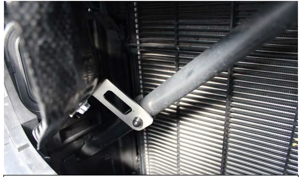
18. Push the clip onto the strut brace.
