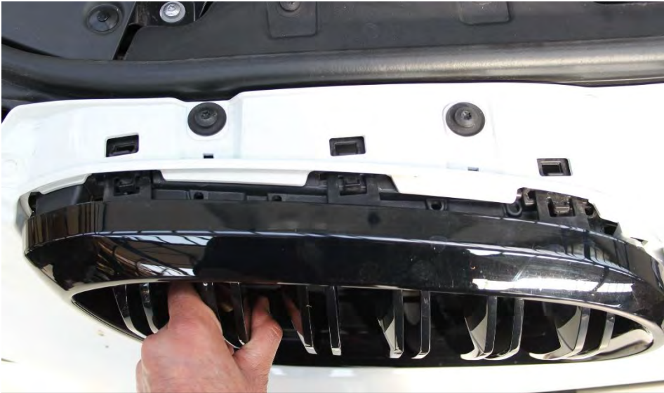
13. Remove the grills – push the tabs in on the top while pulling to release them.
