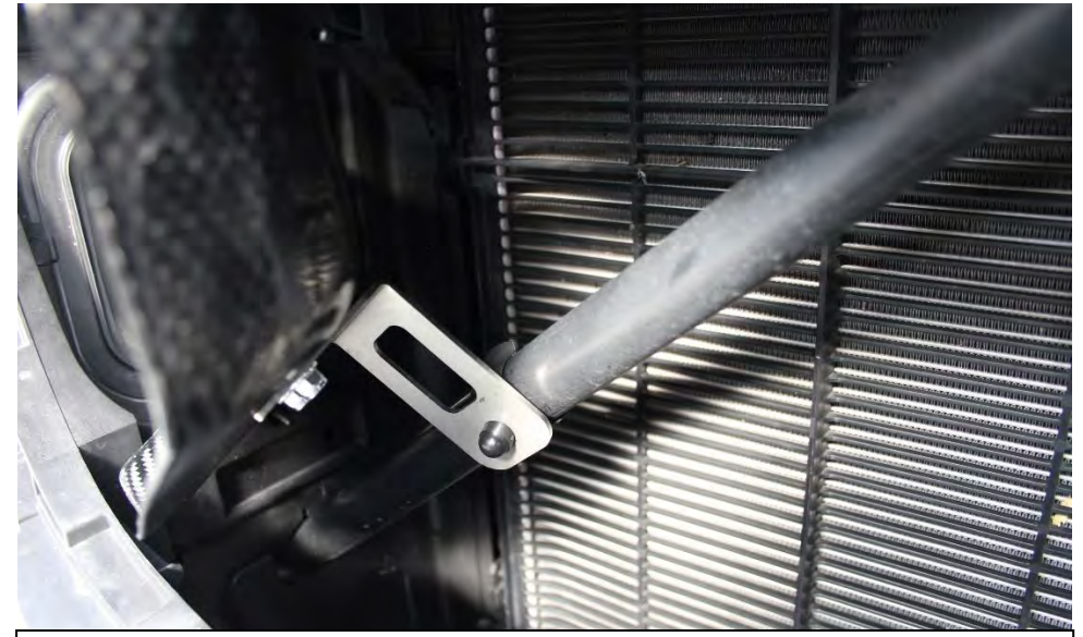
18. Push the clip onto the strut brace.
