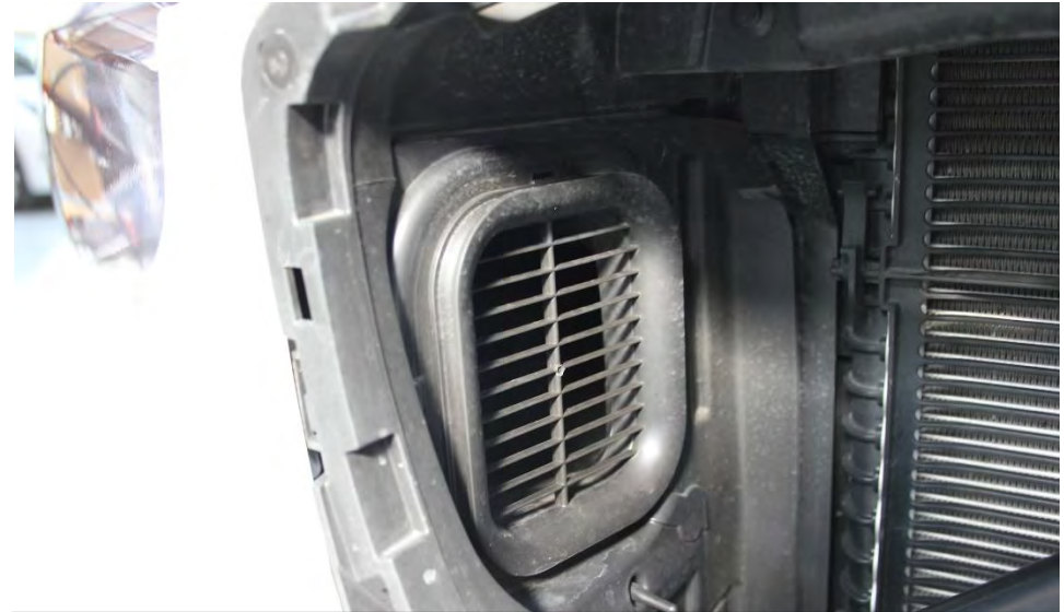
14. Remove the grills covering the air entry ducts.
