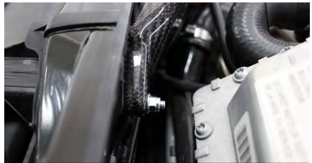
44. Secure with the nut – do not overtighten. Once the duct is unable to move stop tightening.
