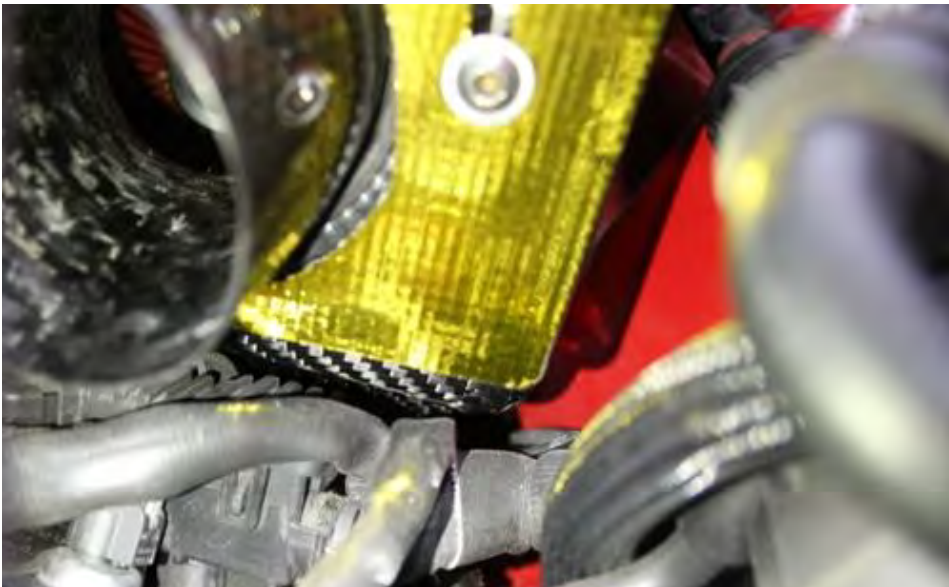
55. Check that the front of the box has a small gap above the plastic loom box.
