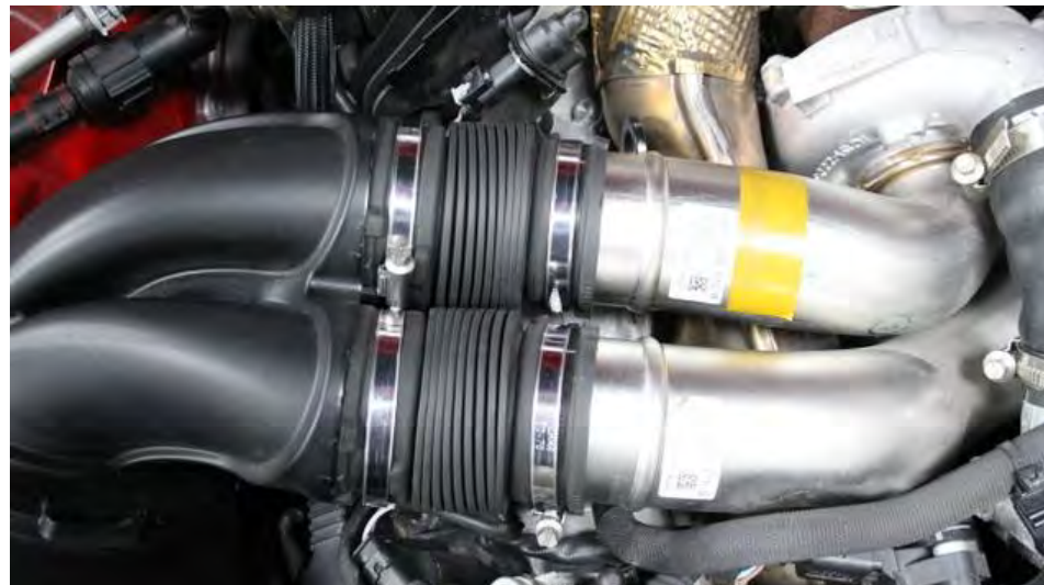
2. Pull the hoses away from the turbo tubes.
