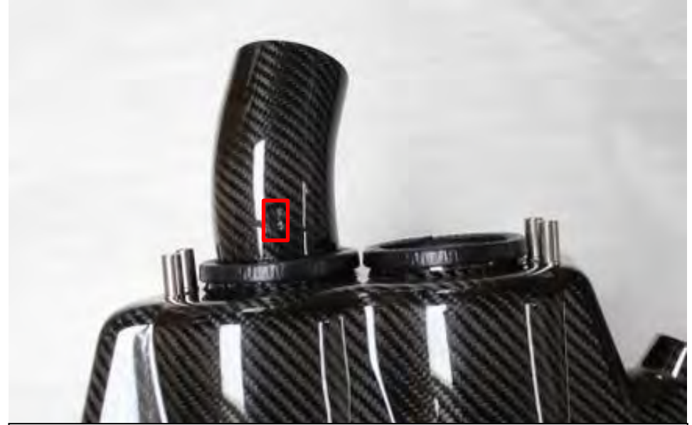
18. Push the tube through the hole and rotate it so you can see the notch in the tube at the top. Shown in red.
