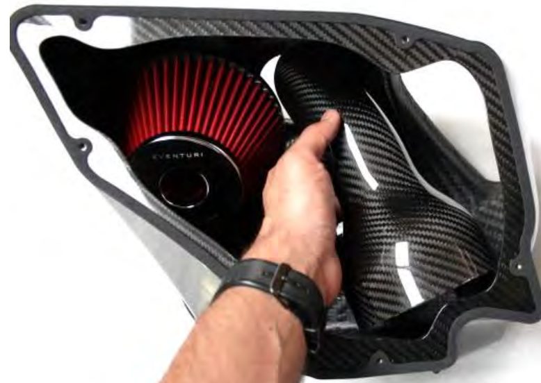
20. Take the longer tube and carefully place into the airbox – push the tube through the hole.
