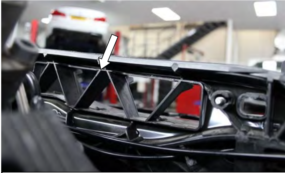
37. Ensure that the carbon duct top edge as highlighted in red previously, goes above this edge shown here.
