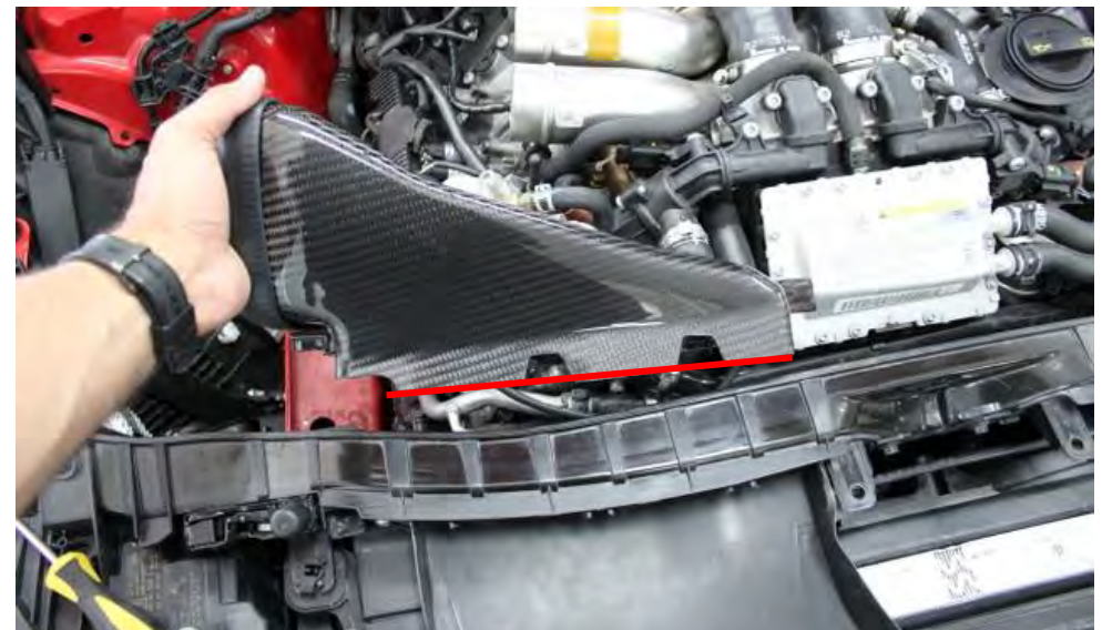
36. Take the carbon duct and position into place. Notice the top edge highlighted in red - see next steps for details.
