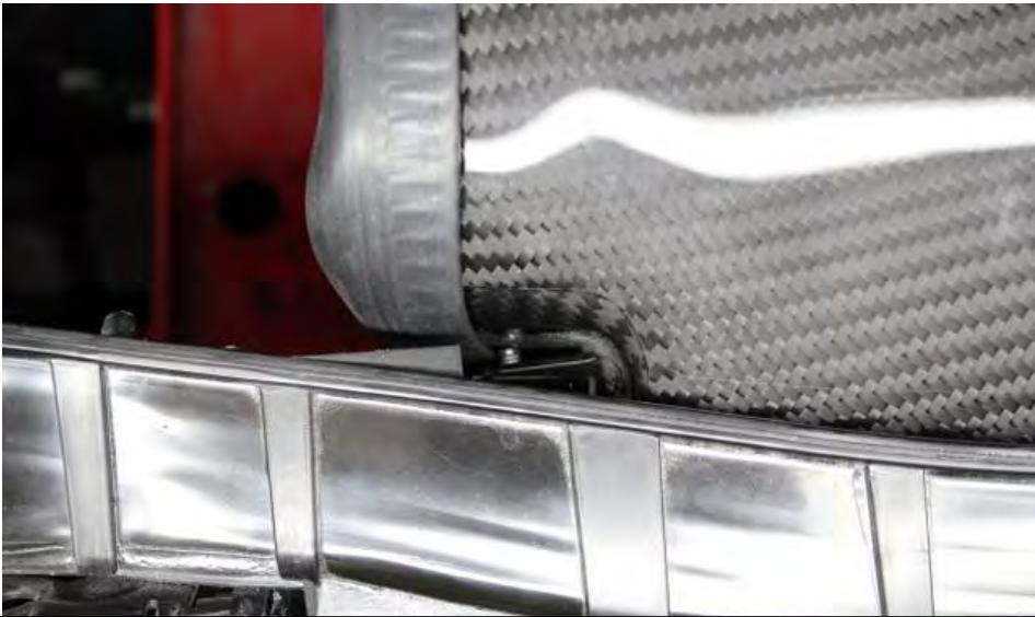
41. Secure the left side closest to the rubber edging with the OEM screw. Do not let the screw contact with the carbon.
