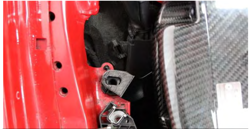
54. The rear bracket from the airbox should line up with the remaining rubber mount. Before securing this – check the clearance in the next step.
