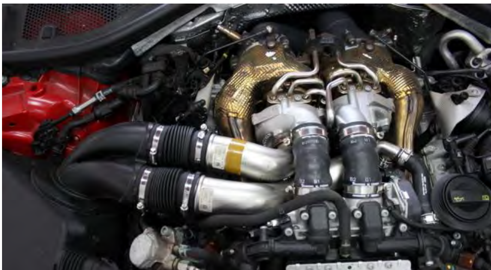
1. Remove Engine cover and loosen the clamps around the inlet hoses of the airbox.
