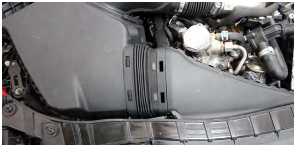
3. Release the flexible connection between the airbox and the duct by pushing the tabs in and pulling the connector out from the duct. The airbox can now be fully removed from the engine bay by pulling it upwards. Make sure to remove the rubber airbox outlet hoses too (from step 2)
