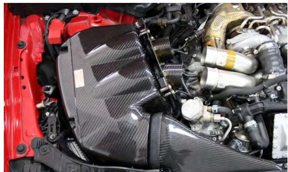
48. You should be able to feel the second mount also going into the hole in the chassis. The airbox should line up as shown with the duct. We will seal it with the rubber on the duct later.
