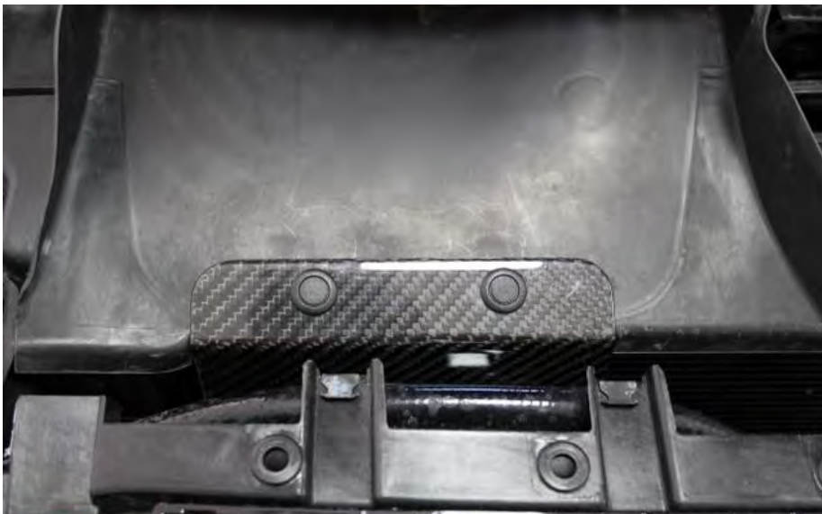
35. Re-position the scoop and secure with the 2 x 6mm plastic rivets as shown.
