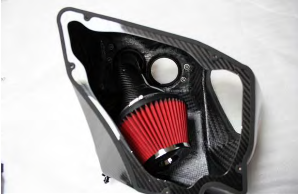
17. Push the carbon tube through the left hole in the airbox as shown.
