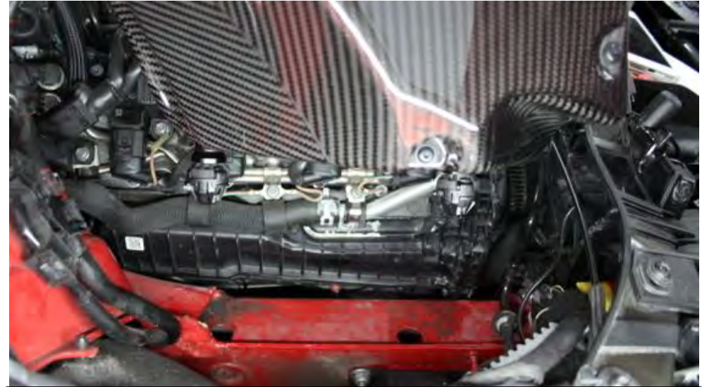
46. Now take the airbox and carefully lower it into the engine bay – guide the 2 mounts towards the holes in the chassis.
