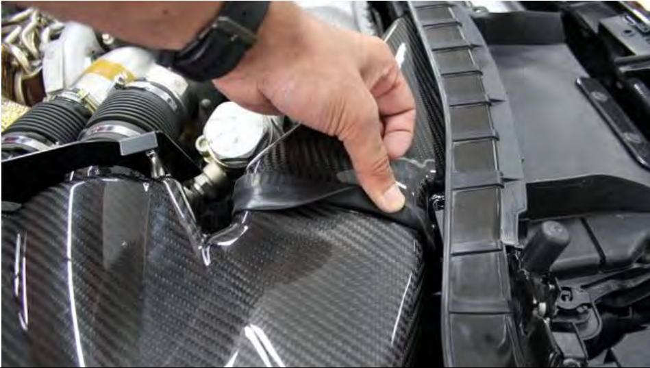
53. Now pull the rubber on the duct back and position the airbox inside the rubber.
