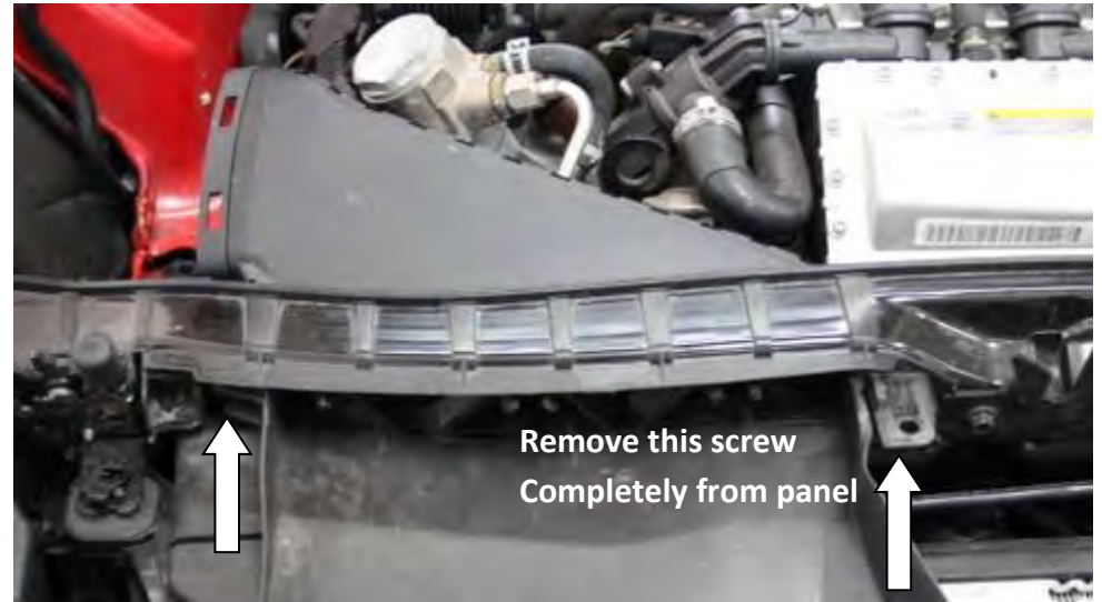
14. Now remove the duct by unscrewing 2 torx screws as indicated. You need to completely remove the right side screw. Left one can be left in place.
