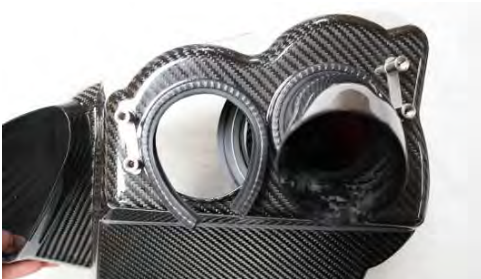
19. For the remaining tube – first remove JUST the lower parts of the rubber edging from the airbox as shown.
