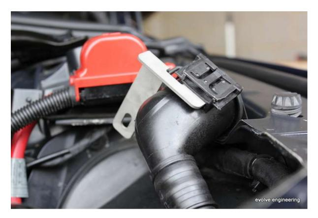
26. Secure bracket to right side panel using supplied flanged bolt and nut as shown:
