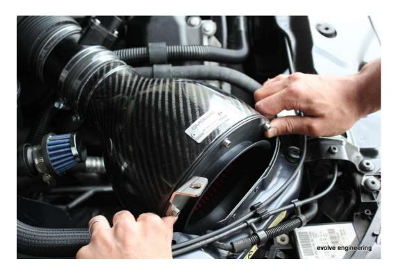
iii. You may need to rotate the assembly to align the bracket to the bush
