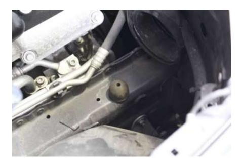
iii. Install heat deflectors behind air feed and align holes making sure you locate lower bracket onto chassis thread:
