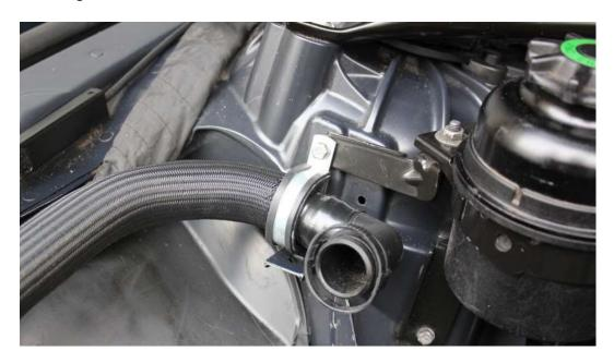
22. Push in supplied breather filter assembly into the secondary air pump tube. This will click into position:
