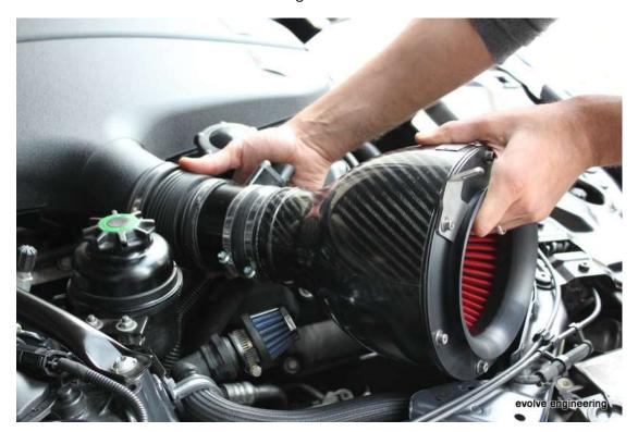
ii. Compress the assembly and lower the intake onto the locating bush through the bracket hole. We have supplied a spare bush if required.
