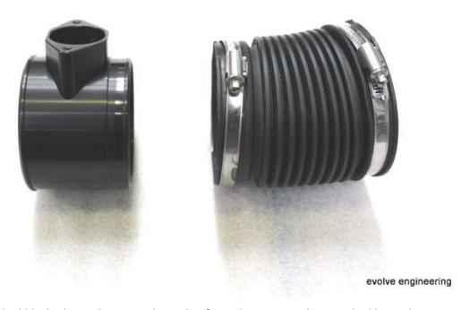
12. Fit supplied black silicone hose to other side of MAF housings with 2 supplied hose clamps (Please ensure silicone hose is straight on the MAF housing and touching the MAF boss – see image)
