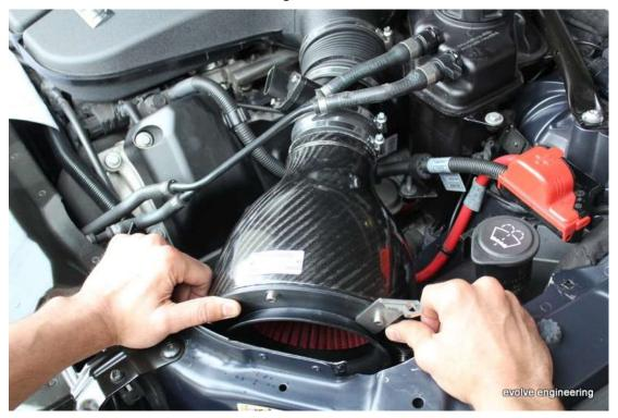
iii. Compress the assembly and lower the intake onto the locating bush through the bracket hole (see picture)
