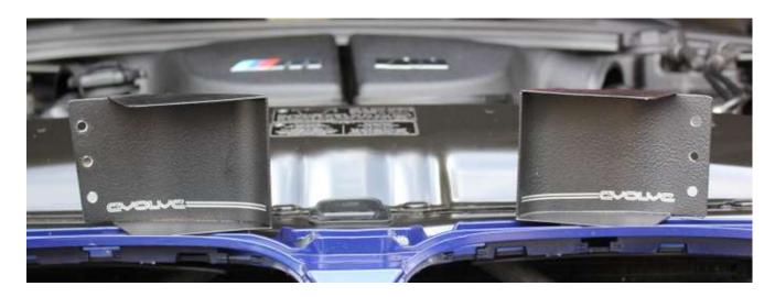
19. Drill 2mm pilot holes with scoops in place and secure with supplied screws:
