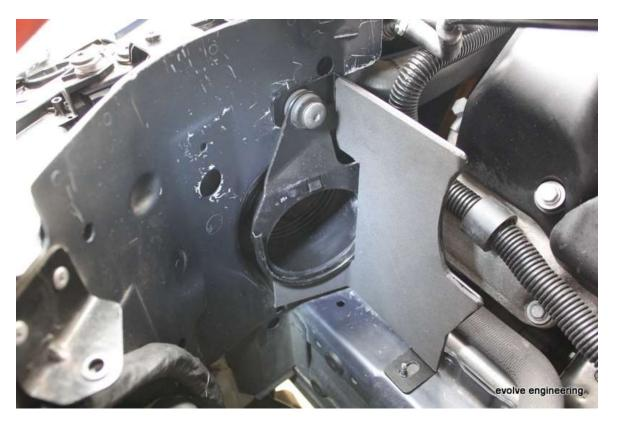
iv. Secure with OEM torx through the air feed and supplied plastic nut or existing rubber bush onto chassis
