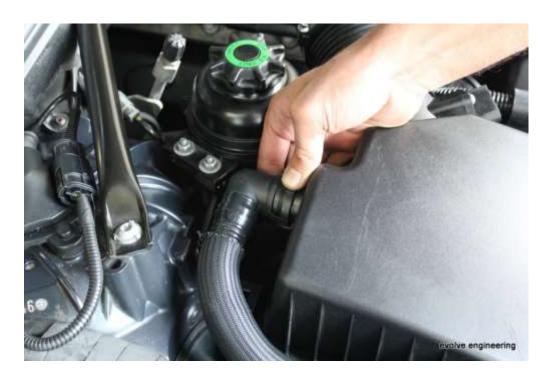
3. Remove upper airbox assemblies by unclipping latches and loosening hose clamps complete with flexible tubing to inlet manifold
