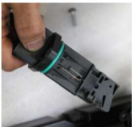
10. Insert MAF sensors into Evolve MAF housings using supplied bolts Tighten bolts to maximum 5Nm
