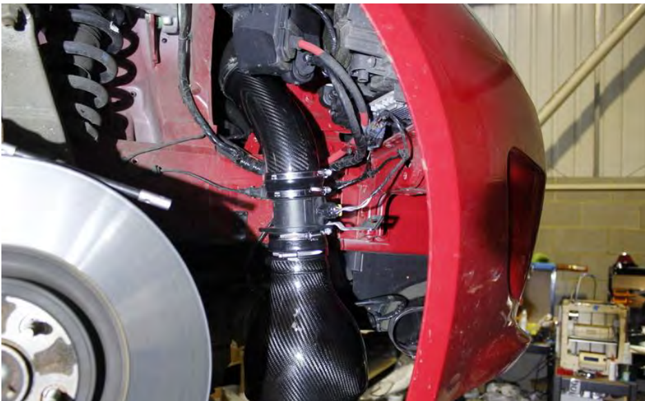
27. As previously, push the carbon tube into the stock plastic intake tube and then the housing.
