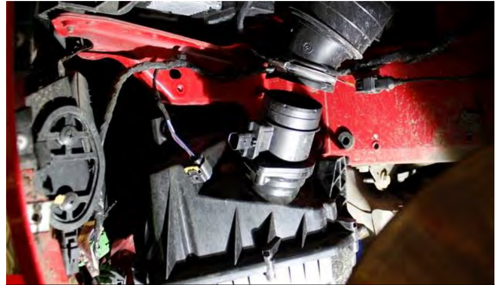
6. Pull the airbox out of position and remove completely from the arch.
