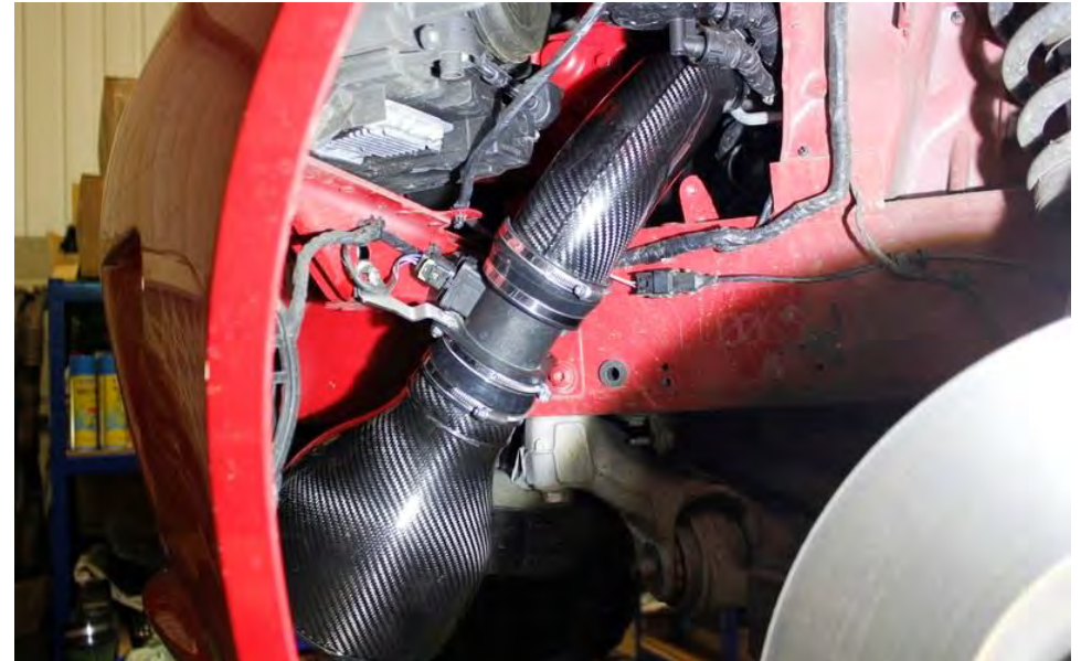
18. Rotate the entire assembly as shown so that the housing goes into the arch and the bracket lines up with the mounting hole shown above and in the next step. You may need to rotate the MAF tube also.
