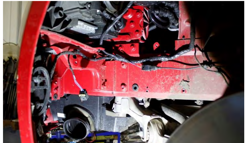
8. Here is the airbox and short tube removed.
