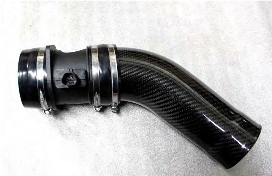
25. Using the relevant silicon hoses – assemble the remaining carbon tube to the LHS MAF tube as shown.
