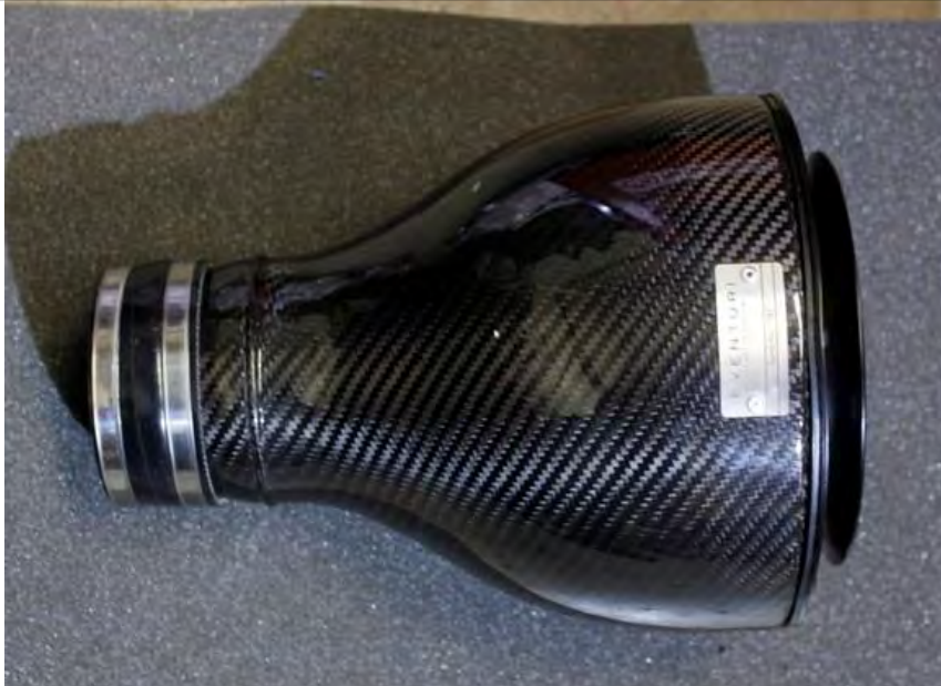
15. Assemble the relevant silicon hose to one of the filter housings. You may also assemble this hose onto the other side of the MAF tube if it is easier for you.
