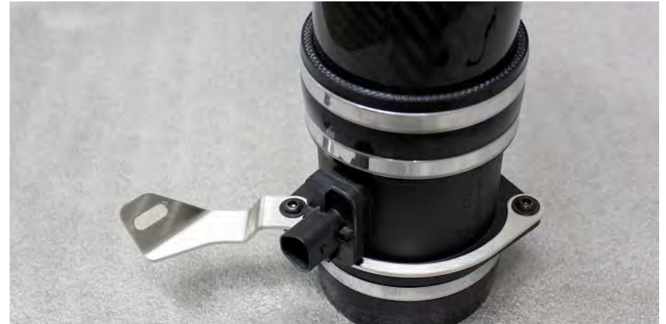
14. Secure the RHS bracket to the MAF tube as shown. Here we are showing the V8 version. The V6 version attaches in the same orientation. Use the supplied bolts and locking nuts.
