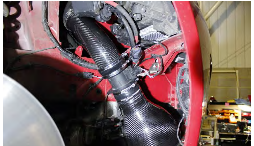
28. Rotate the assembly and line up the bracket to the mounting point on the chassis.
