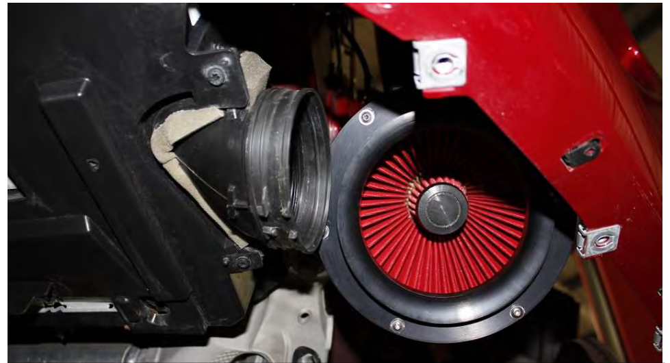
20. The opening of the housing should be positioned as shown over the stock duct. Once lined up and secured, tighten all the hose clamps – do not overtighten.
