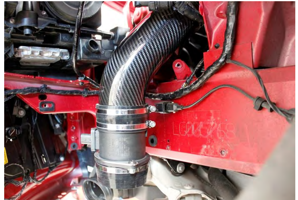
16. Push the carbon tube into the stock plastic intake tube – it is a tight fit but it will push into the plastic tube. Be careful of any protruding clips around the stock tube – they may scratch the carbon. Point the tube downwards as shown. Do not tighten the upper hose clamp yet.
