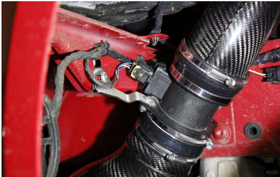
19. Line up the bracket with the mounting hole and secure with the supplied M6 bolt. Insert the MAF sensor plug back into place fully.
