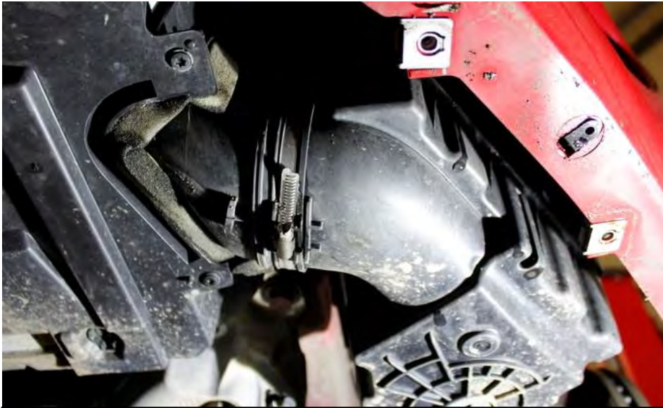
5. Loosen hose clamp at the base of the airbox holding the duct feed in place.
