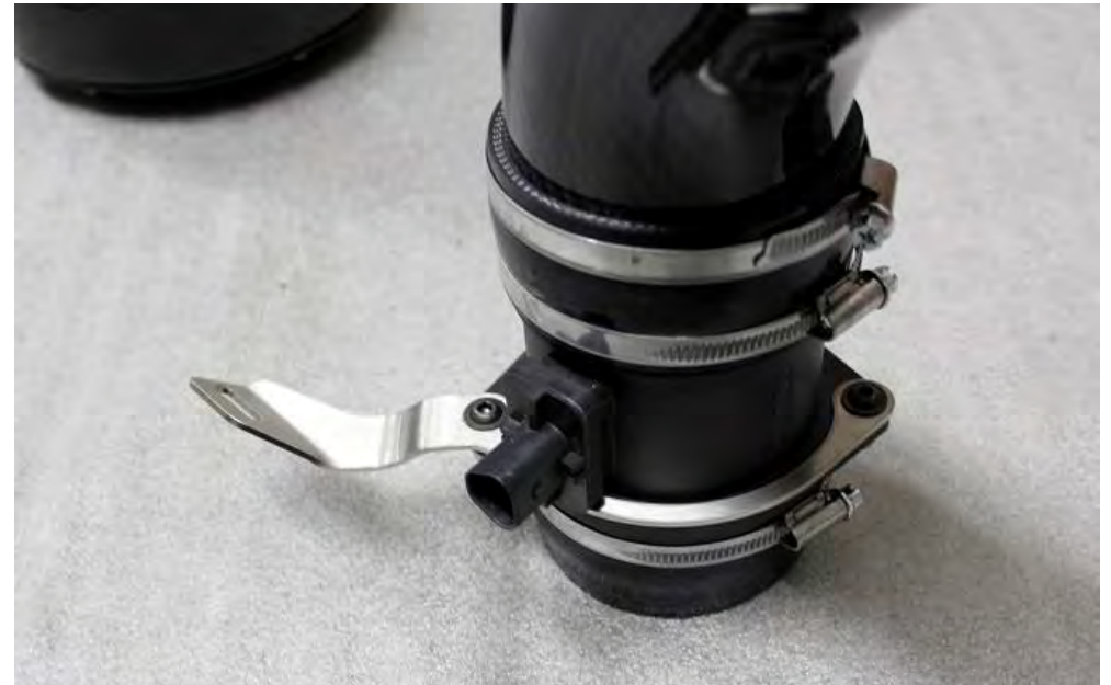
26. Install the remaining bracket as shown using the supplied bolts and lock nuts.
