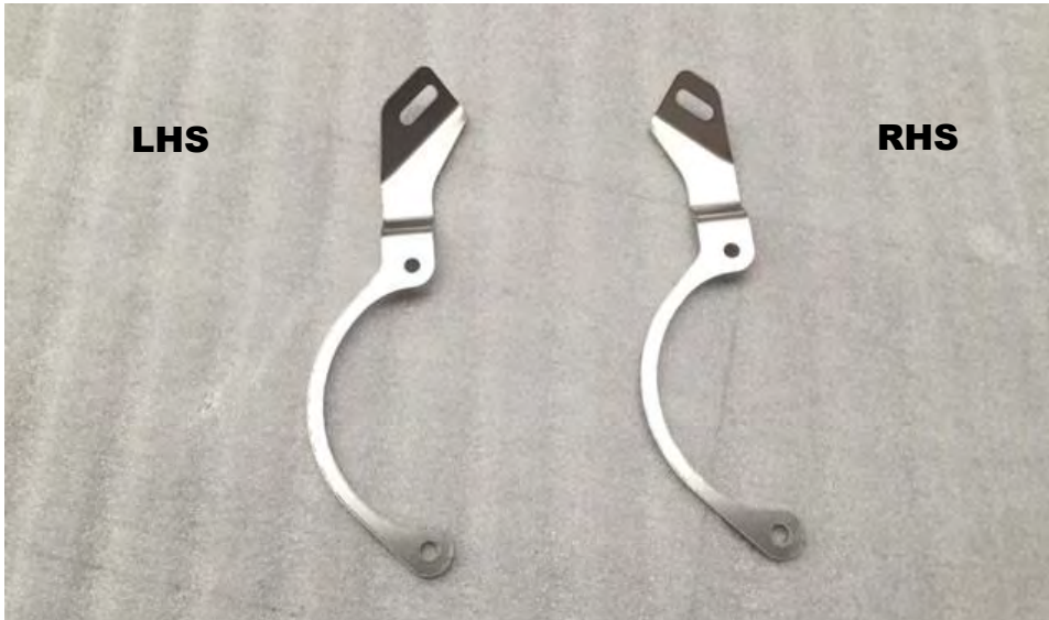
13. Here are the LHS and RHS V8 brackets used to secure the MAF tube to the chassis. The V6 versions don't have the half circle portion.
