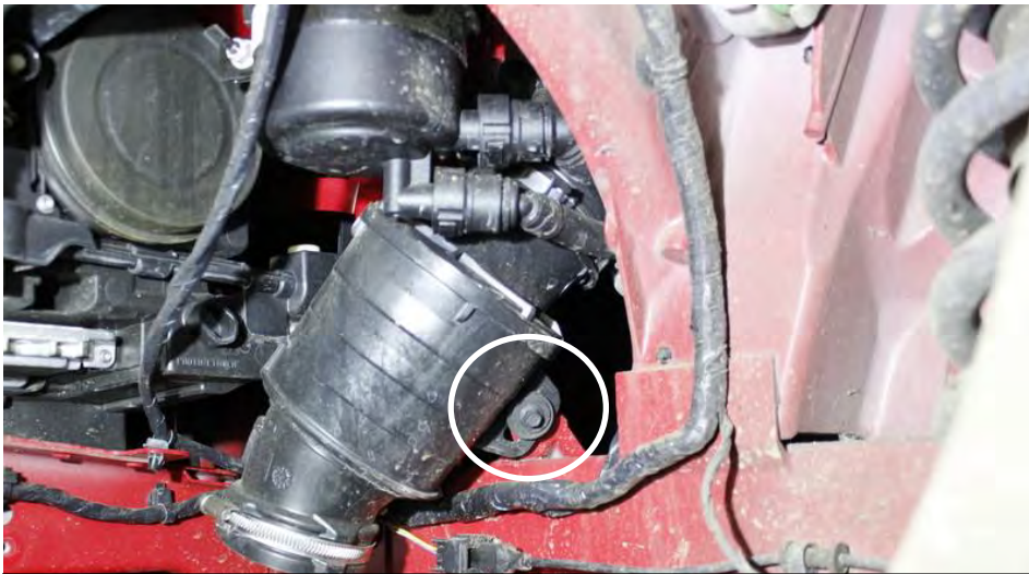
7. Now remove the short inlet tube – there is a bolt to remove as shown and also a hose clamp at the top to loosen. This connects the tube to the longer intake tubes – not shown in the photo.
