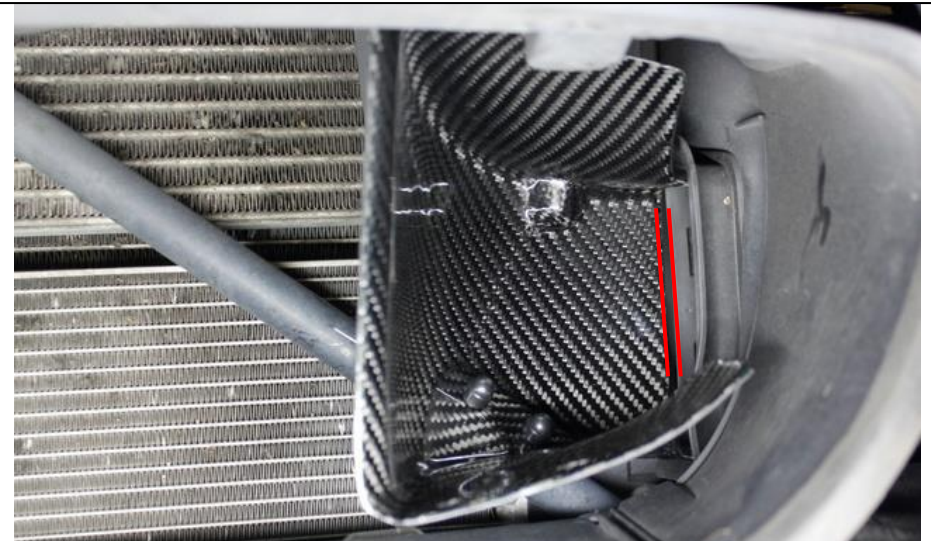
12. The scoop should sit as shown here. Notice the scoop outlet is lined up with the stock duct entry highlighted in red.
