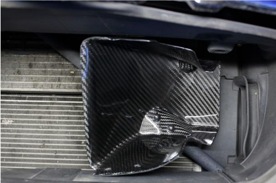
9. Push the scoop all the way back and push the clamps at the back of the scoop onto the strut brace.
