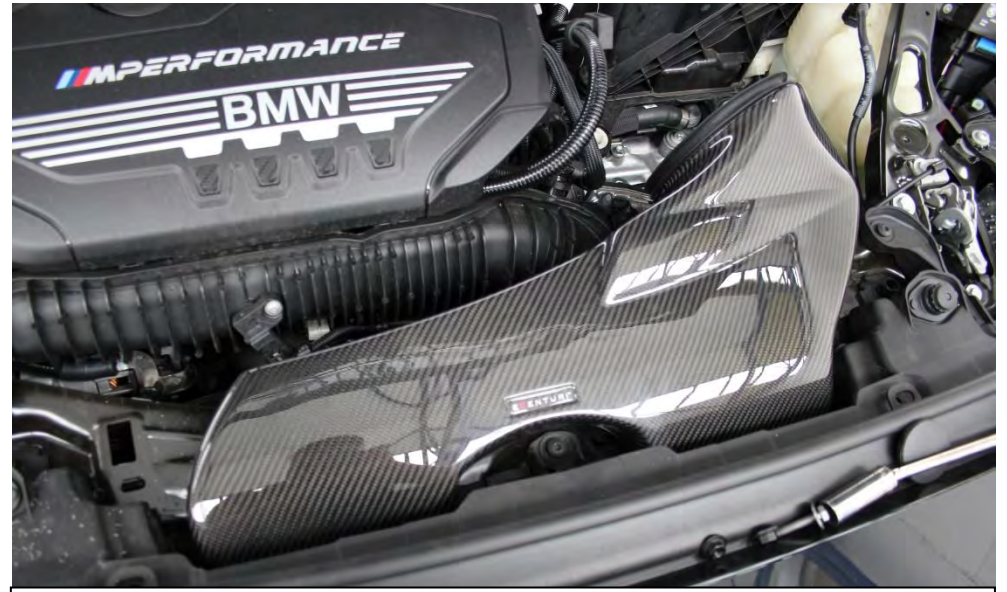
10. Install the duct into place.
