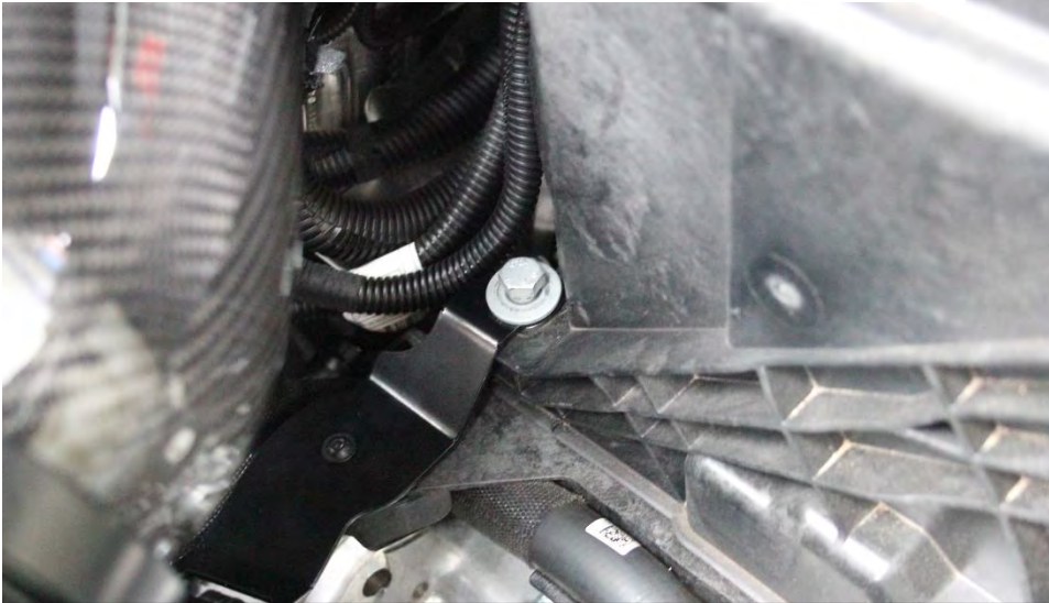
17. Secure the housing bracket with the bolt removed previously.
