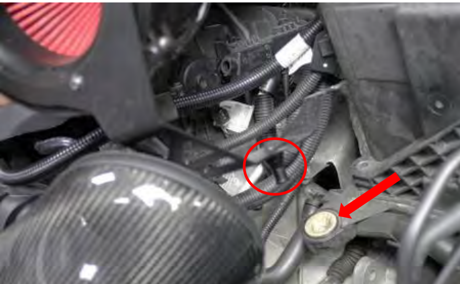
15. At the base of the bracket on the housing there is a mounting locator (circled) – push this into the rubber grommet indicated by the arrow.
