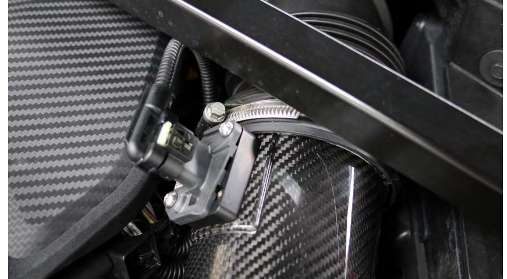
18. Reconnect the MAF plug and secure the hose clamp around the inlet tube. Do not over tighten.
