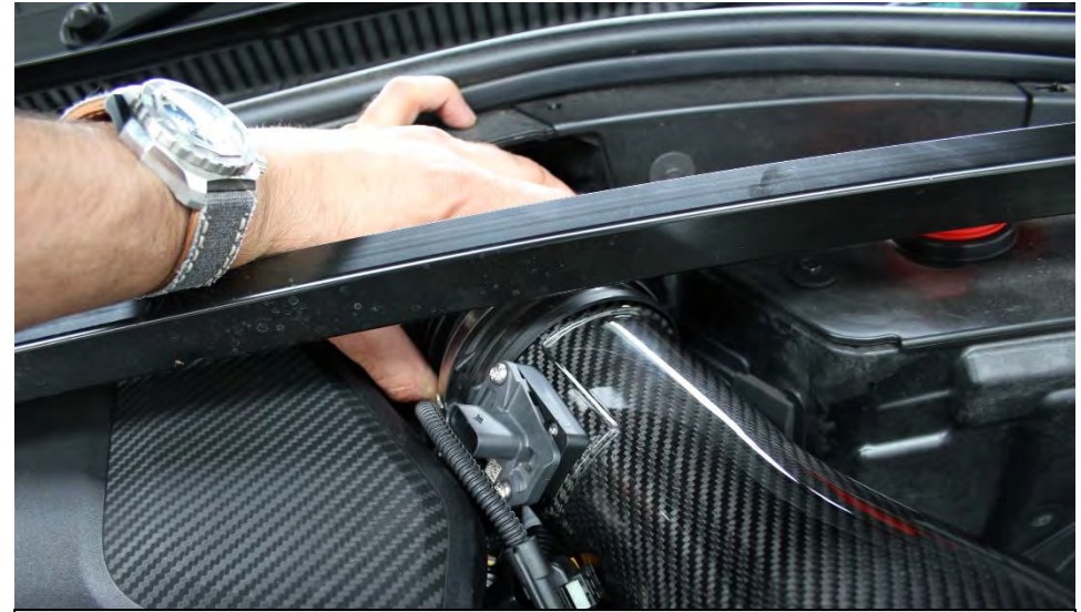
14. Push the filter housing into the turbo inlet pipe. Make sure it is all the way in. The pipe should almost touch the MAF sensor holder.
