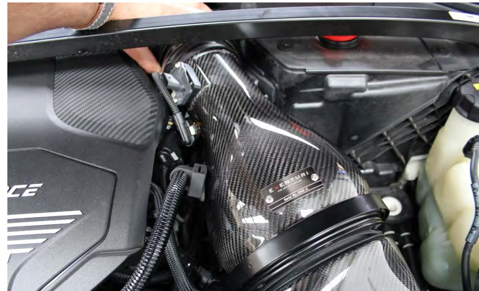
16. Line up the filter housing with the duct and then secure the bracket with the Bolt removed previously. See next step.
