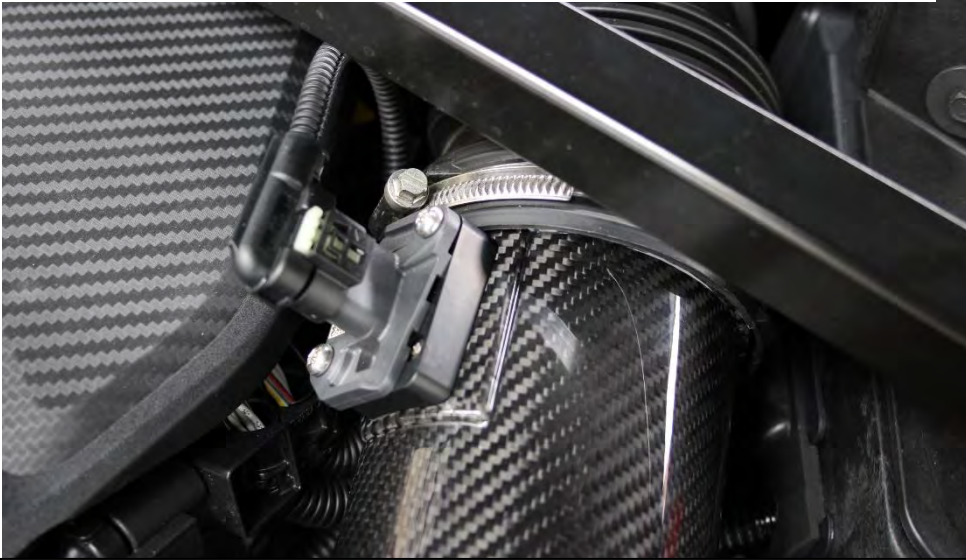
21. Reconnect the MAF plug and secure the hose clamp around the inlet tube. Do not over tighten.
