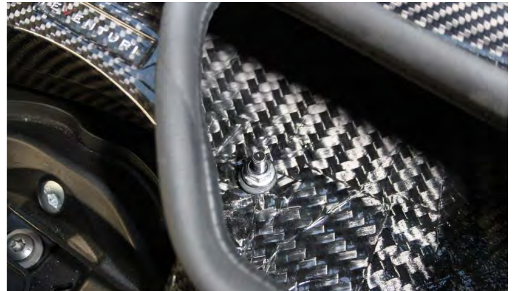
16. Secure the duct through the openings with the nuts removed in step 2.
