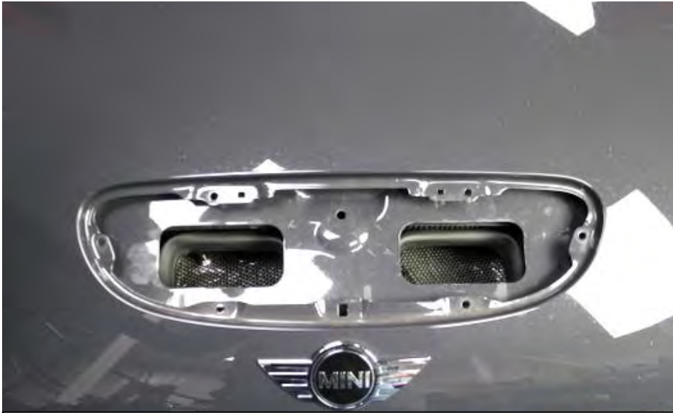
25. With the scoop removed – the clip locations can be seen on the bonnet ready for the carbon scoop.
