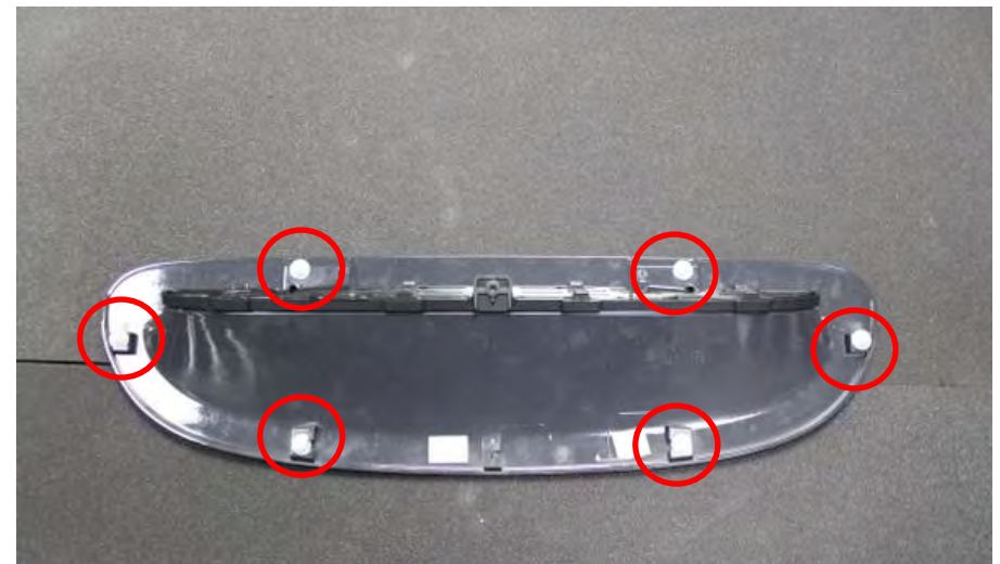
24. Here is the back of the scoop and the clip locations.
