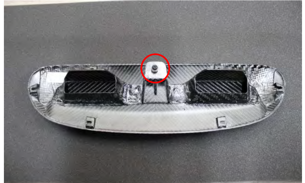
26. Check the back of the carbon scoop – if you have an M5 screw pre-installed as shown then remove it. If not - simply continue to the next step.
