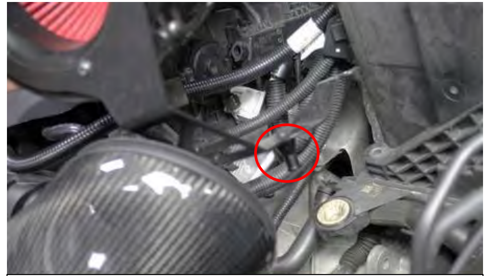
18. At the base of the bracket on the housing there is a mounting locator (circled) – push this into the rubber grommet indicated by the arrow.
