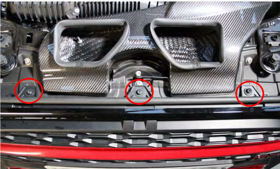
15. Secure the bumper with the 3 Torx screws removed previously.
