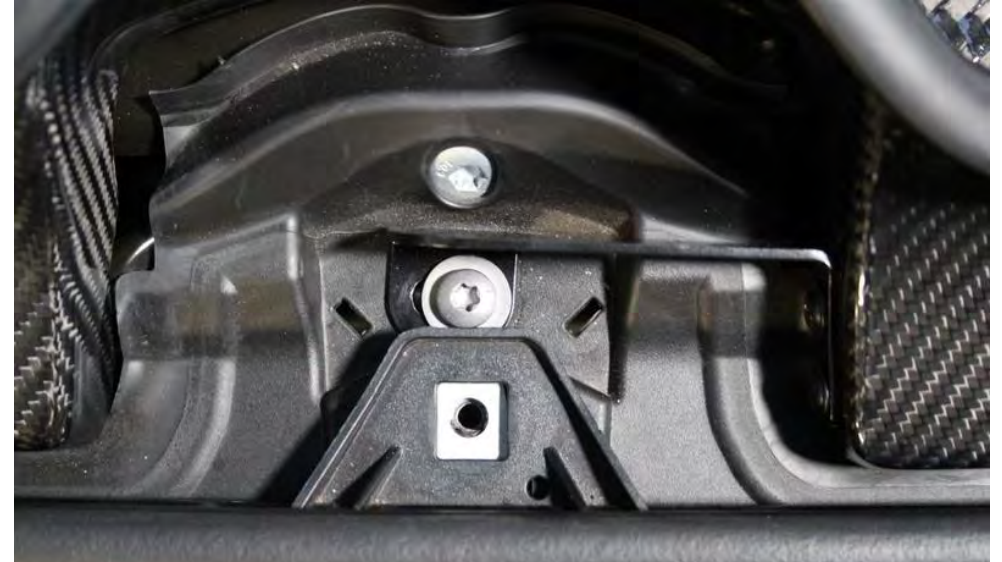
14. Secure the middle bracket with the Torx screw removed previously.
