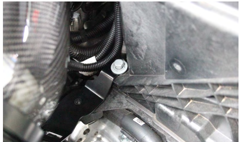
20. Secure the housing bracket with the bolt removed previously.
