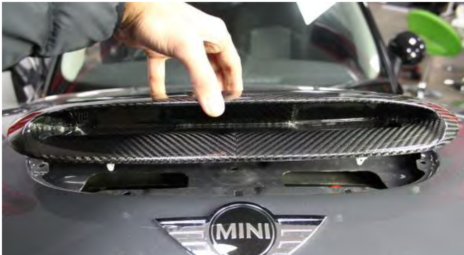
27. Carefully lower the carbon scoop into position – make sure the 6 clips are already installed on the back of the scoop.
