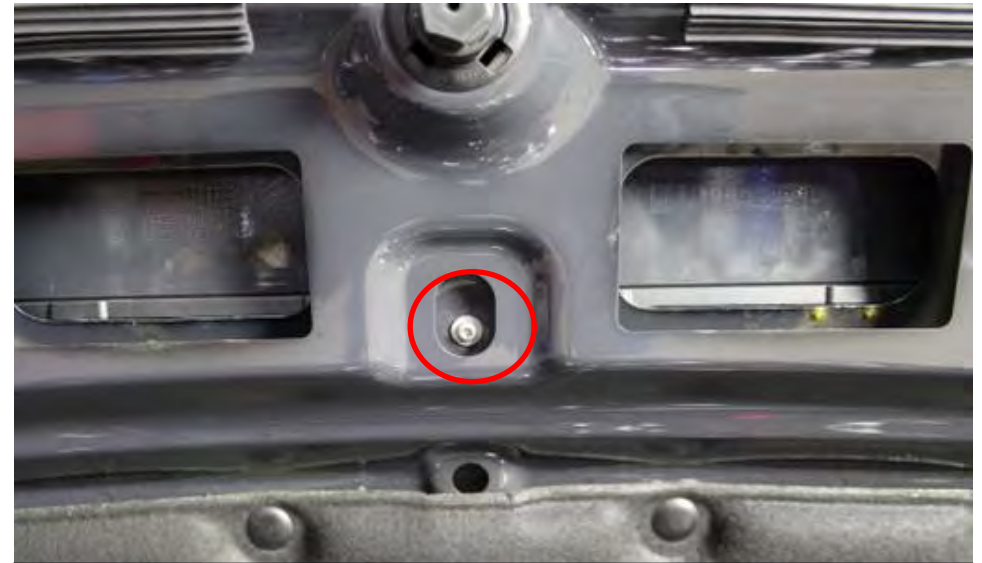
22. Now we will remove the bonnet scoop. Start by removing the torx screw shown.
