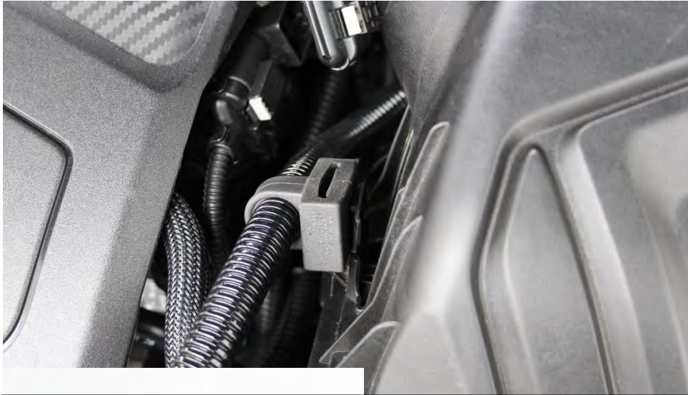
5. Remove the rubber loom holder from the left side of the airbox.
