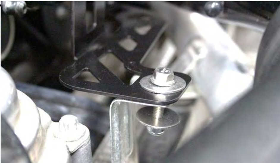
15. Insert the screws through each bracket and through the stock airbox mounts. The washers should be on each side as shown. Don't tighten yet.
