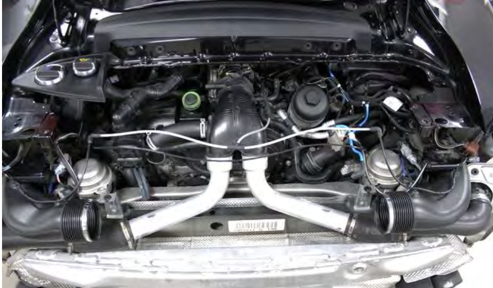
9. Loosen the 2 hose clamps on each side of the airbox at the outlets and then the airbox can be removed from the engine bay.
