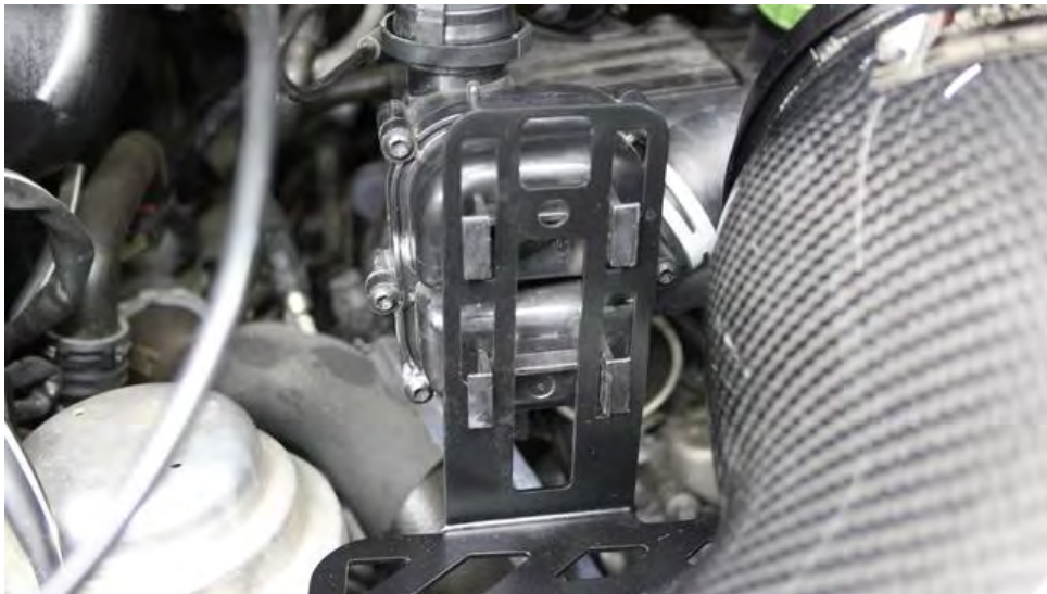
11. Slot the left side module into the bracket as shown.
