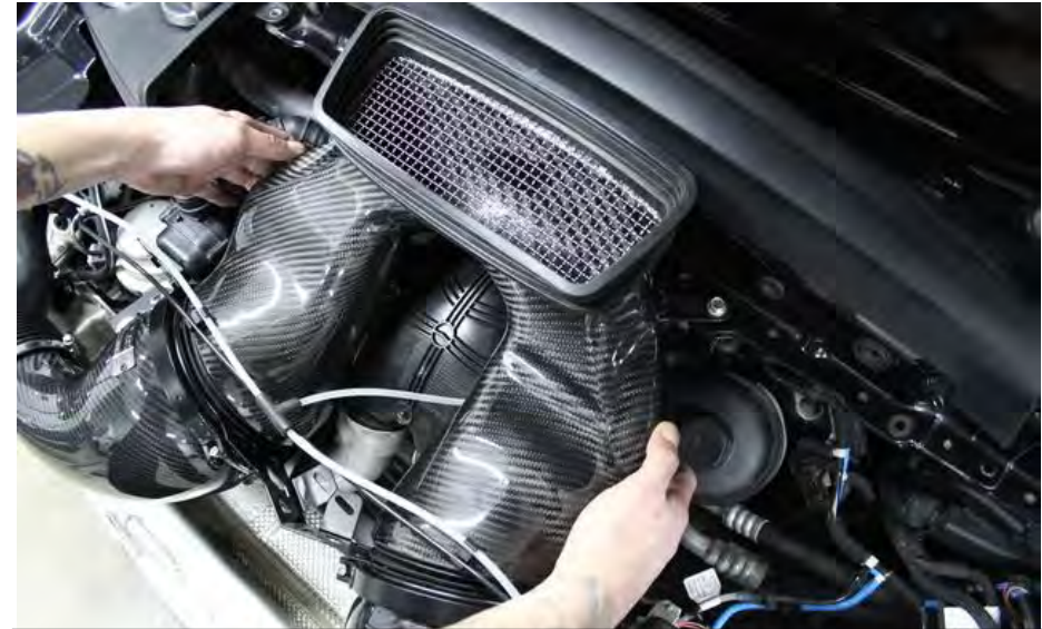
30. You will need some help for this step – the duct needs to be pulled forwards so that the rubber seals compress onto the filter housings.
