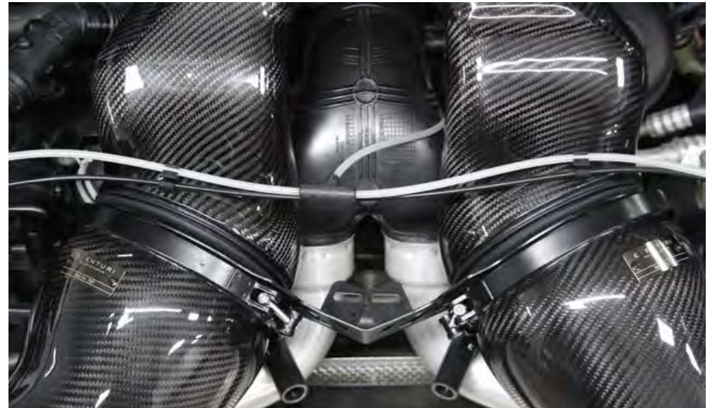
32. The fully secured system should now have a good seal between the duct and the filter housings.
