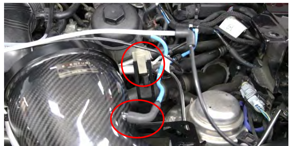
12. Push the right side module onto the bracket and push the vacuum connector into the outlet on the filter housing.
