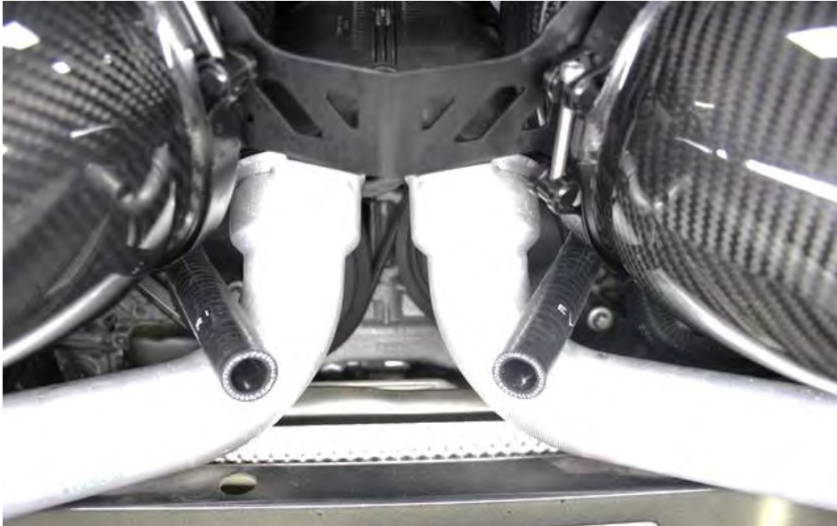
13. Rotate the 2 drain tubes under the filter housings so that they are positioned as shown.
