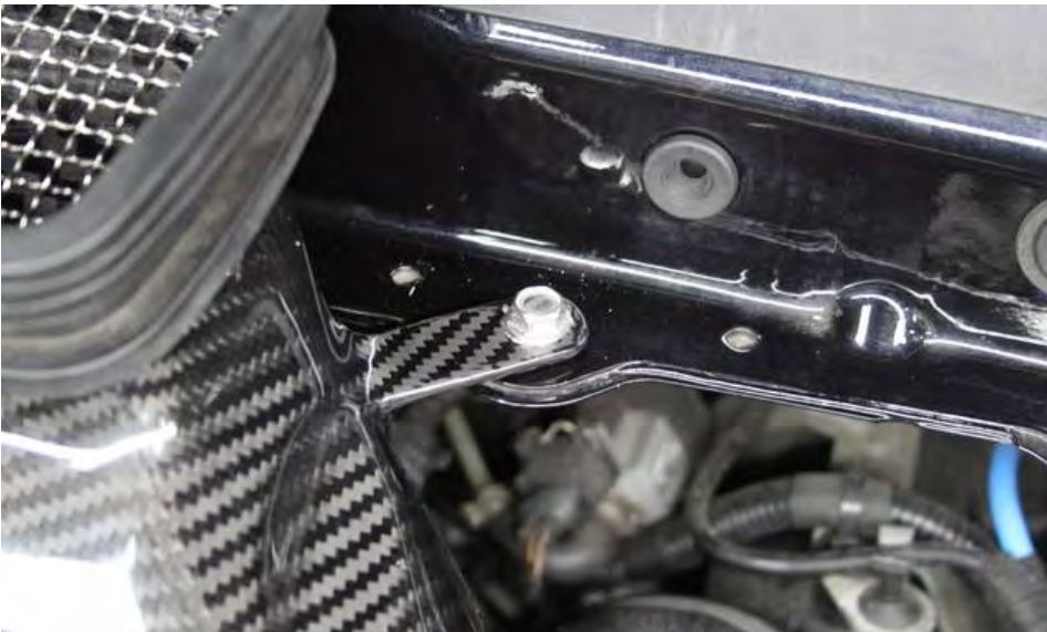
31. While the duct is being pulled forwards – tighten the 2 screws on the mounts to secure the duct into position.
