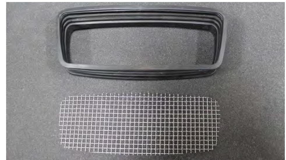
16. Take the stock duct rubber surround and the provided mesh insert.
