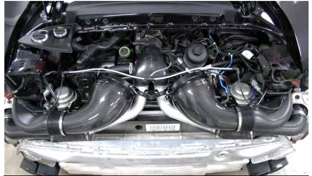
10. Take the filter housing assembly and position the brackets on top of the stock airbox mounts. Push the stock inlet tubes onto each intake housing. Don't tighten yet.
