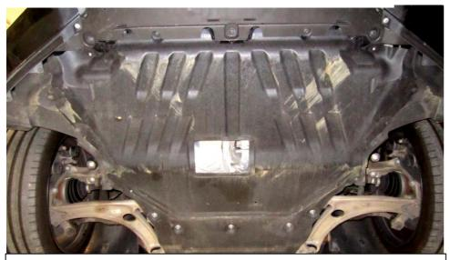
1. We will start with the assumption that the stock airbox has already been removed. Remove the undertray
