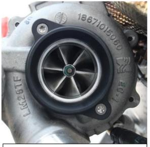
12b. CORRECT – the flange is concentric with the turbo inlet.
