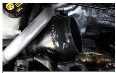
34. For the 3.5" intake, attach the reducer silicon as shown.
