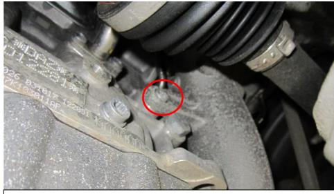
2. Remove the screws which hold the metal boost pipe in place. There are 2 screws as shown here and in the next step.
