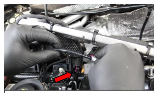
$28. \ Take \ the \ supplied \ vacuum \ line \ and \ connect \ it \ to \ the \ plastic \ vacuum \ connector \ from \ step \ 6.$
