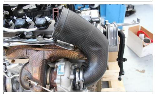
19. Push the inlet tube firmly into the silicon and ensure is it fully in. Do not tighten the clamp yet.
