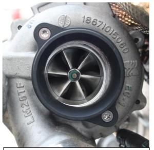
12a. INCORRECT – the flange is not concentric with the turbo inlet. Rotate the flange 180 degrees.
