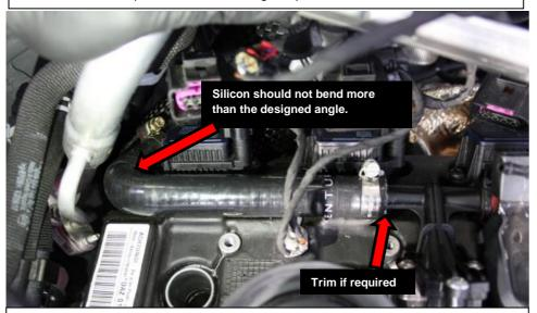
23. The Silicon tube should NOT be forced to bend into position more than it is shaped to be. If this tube is too long it will be forced to bend more than the designed angle and this will stop the breather system from working properly. Trim the silicon tube if required.
