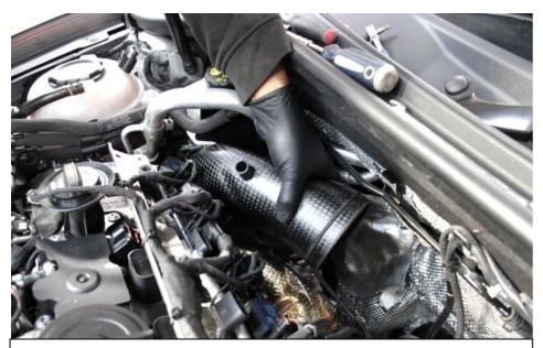
17. Rotate it around the manifold heat shield.
