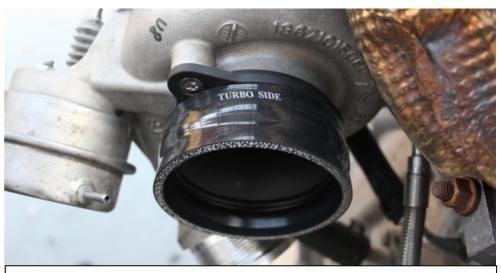
14. Push the silicon onto the flange so that the "TURBO SIDE" writing is closest to the turbo. The silicon will be tight to push on but will snap into place as the bead around the flange locks into the groove inside the silicon.
