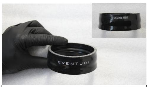
13. Take the small silicon coupler supplied – it has internal grooves. Notice the location of the TURBO SIDE writing.
