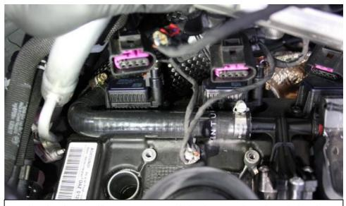
22. Place the adapter and hose into position, push the silicon onto the carbon tube breather inlet. Rotate the carbon tube towards the engine to get the breather assembly into position. The breather adapter should line up with the fixing position on the engine. You may need to trim the silicon tube if it does not.
