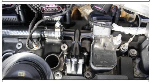
24. Once lined up – secure the plastic breather adapter into place with the 3 torx screws. Also tighten the hose clamp around the silicon tube at this adapter end only. Do not over tighten.
