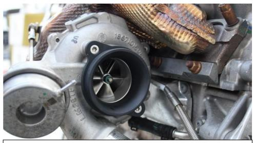
10. Secure the flange to the turbo using the supplied screws – we recommend to also use a thread lock such as Loctite 246. (Photo shown with engine out for clarity).
