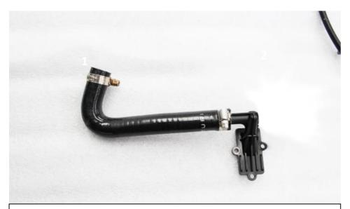
21. Take the Hook shaped silicon tube and attach it to the breather adapter as shown. Use the 2 small hose clamps as shown but don't tighten yet.
