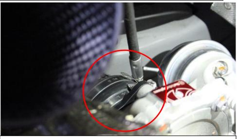
26. Ensure the Carbon tube is still fully engaged in the lower silicon coupler and tighten the hose clamp around the lower silicon. Do not over tighten this with a ratchet. It only needs to be finger tight as the silicon provides a good seal.
