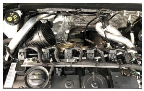
31. Install the coil pack removed previously as well as the loom harness and plugs. Re-attach the undertray.
