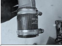
4b. Remove the metal boost pipe.
