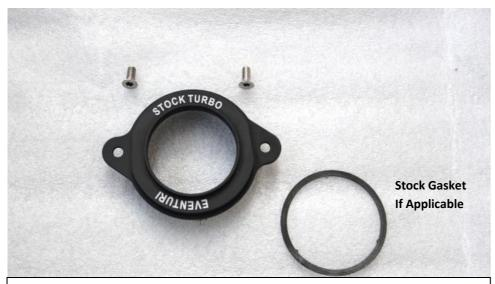
9. Take the new turbo flange with the 2 x countersunk Torx screws. If you are using the stock turbo then you also need to use the stock gasket which may still be on the stock inlet tube.
