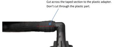
20. Take the oil breather adapter which will still be attached to the stock inlet tube. Carefully cut the tube off the plastic adapter. You just need to make one slit on the tube and it will come off. Be careful not to damage the plastic adapter part.
