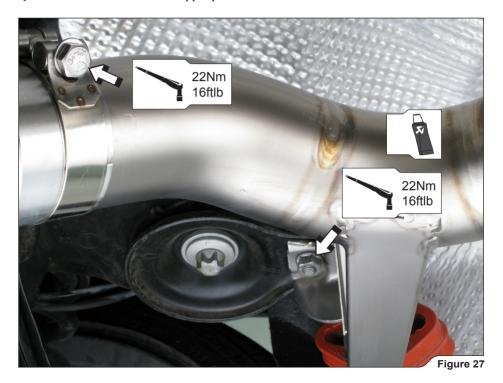
14. For Evolution: tighten to specified torques all bolts and nuts at stock down pipe - Akr. front pipes joint and Akr. front pipes' bracket (Page 20, 21; Figure 13, 14). Adjust the stock down pipe together with Akrapovičt pipes so, that the pipes don't touch any part of the vehicle (there should be at least 10mm gap at any point), than tighten the stock down-pipes' bracket to a specified torque (Figure 28).
