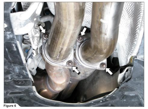
5. For Evolution: unscrew the marked bolts and nuts (Figure 7).
