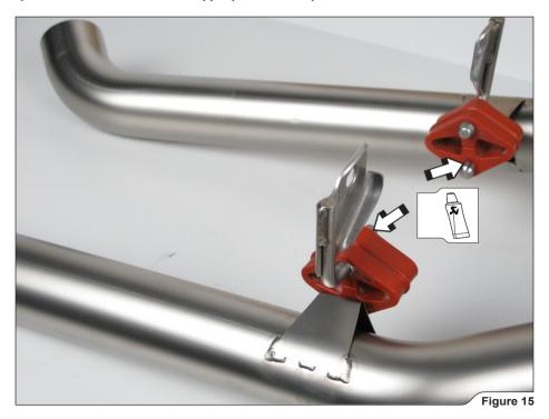
INSTALLATION TIP: coat the interior of the inlet bushes of the middle pipes with ceramic grease (white tube).
