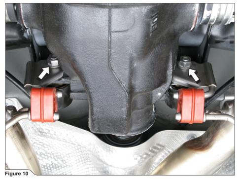
8. **For Evolution:** untighten the marked nuts of the stock down-pipes' bracket, so it can be adjusted later (**Figure 11, 12**).
